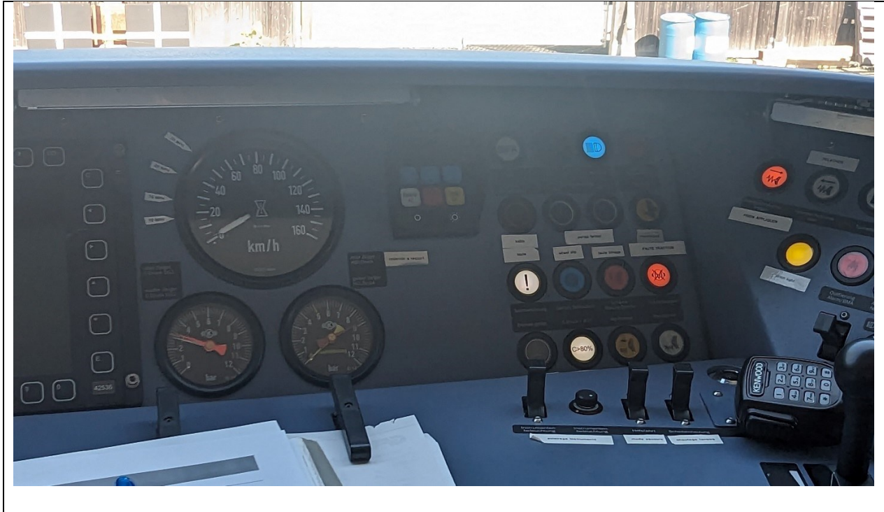
Figure 6: iLint operator station
