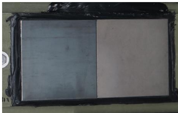
Figure 5-5. Typical surface condition of the bare weathering steel materials utilized in the monitoring array, illustrating the 2.0 mm (left) and 1.18 mm (right) variants.
