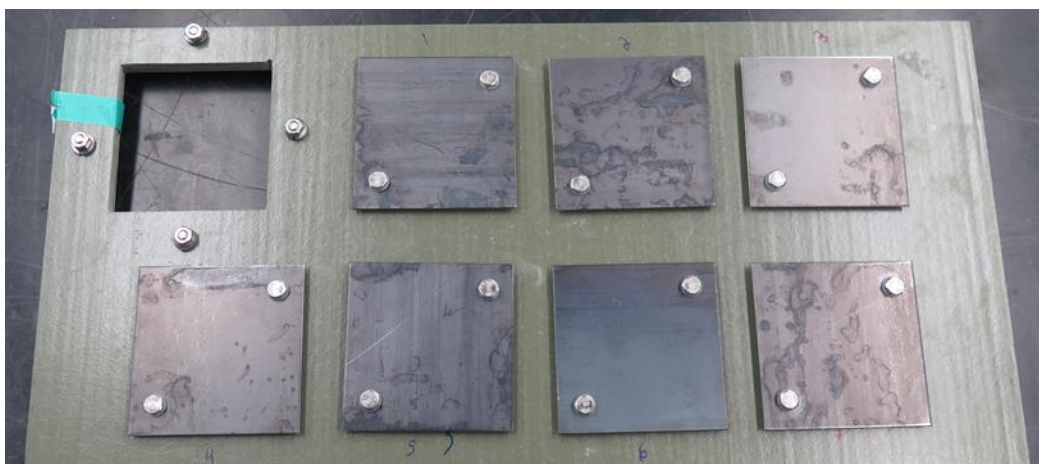
Figure 5-8. Configuration of the weathering steel mass-loss coupons mounted on the side rail plate. This physical array implements the staggered exposure matrix designed to systematically evaluate the influence of discrete seasonal environmental variations on the structural corrosion kinetics.
