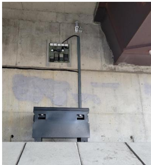
Figure 5-21. Detailed view of the right abutment wall. This installation includes Plate 1, positioned vertically to serve as a baseline monitoring site, and an integrated T/RH sensor for local atmospheric data collection. On the flat surface against the abutment wall is positioned the weather-resistant enclosure that houses the system batteries and the main datalogging hardware. Cables are neatly routed and protected, ensuring long-term structural monitoring and continuous data transmission from this central hub.
