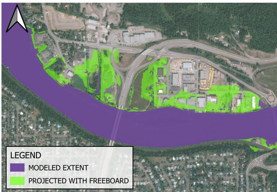
Figure 5-10: Fraser River “protected” areas: projection past berm.
