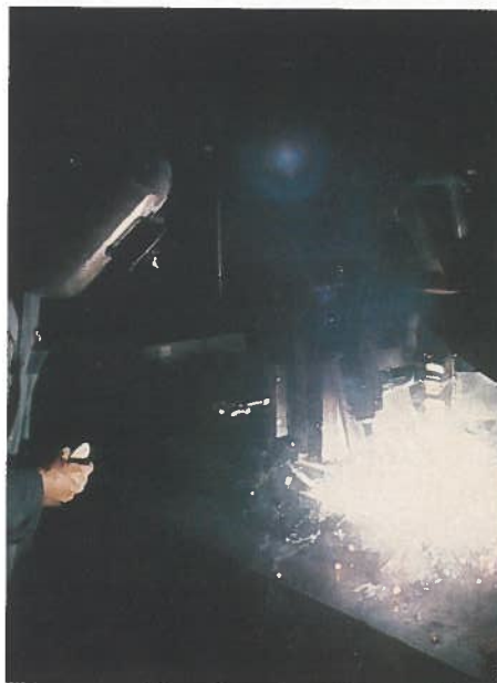
Pulsed MIG welding of aluminum.
