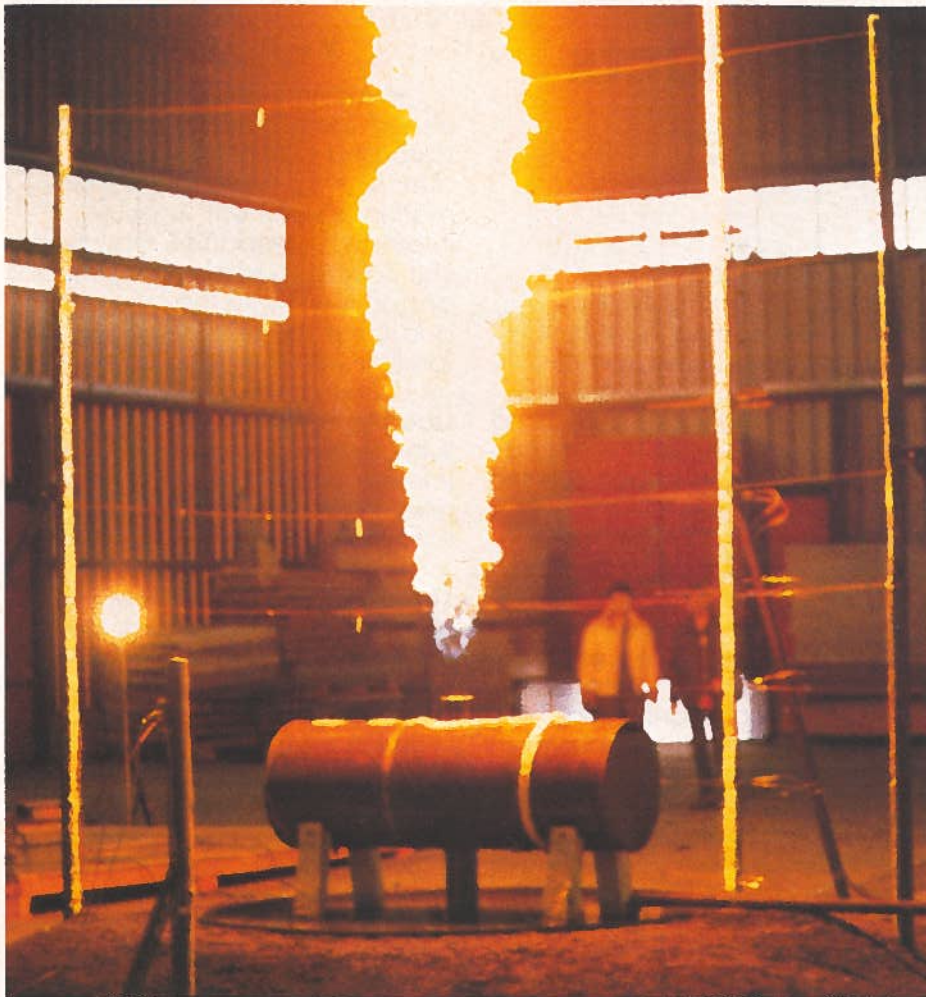
An experiment to simulate venting a propane tank car.
