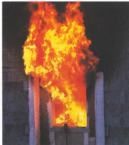
Experiments study the effects of insulation on fire severity.
