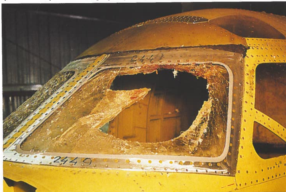
Aircraft windshield damaged by a bird impact.
