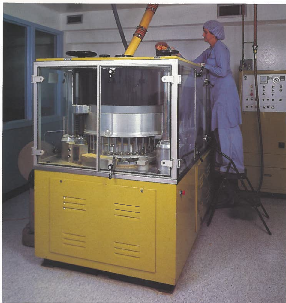
This MG capsulating machine can produce up to 100 000 capsules per hour.
