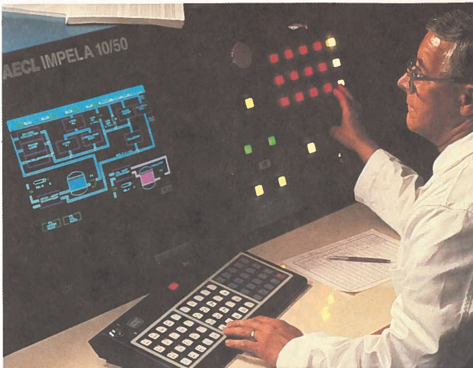
IMPELA's standard industrial programmable logic controller provides automatic start-up and performance monitoring.
