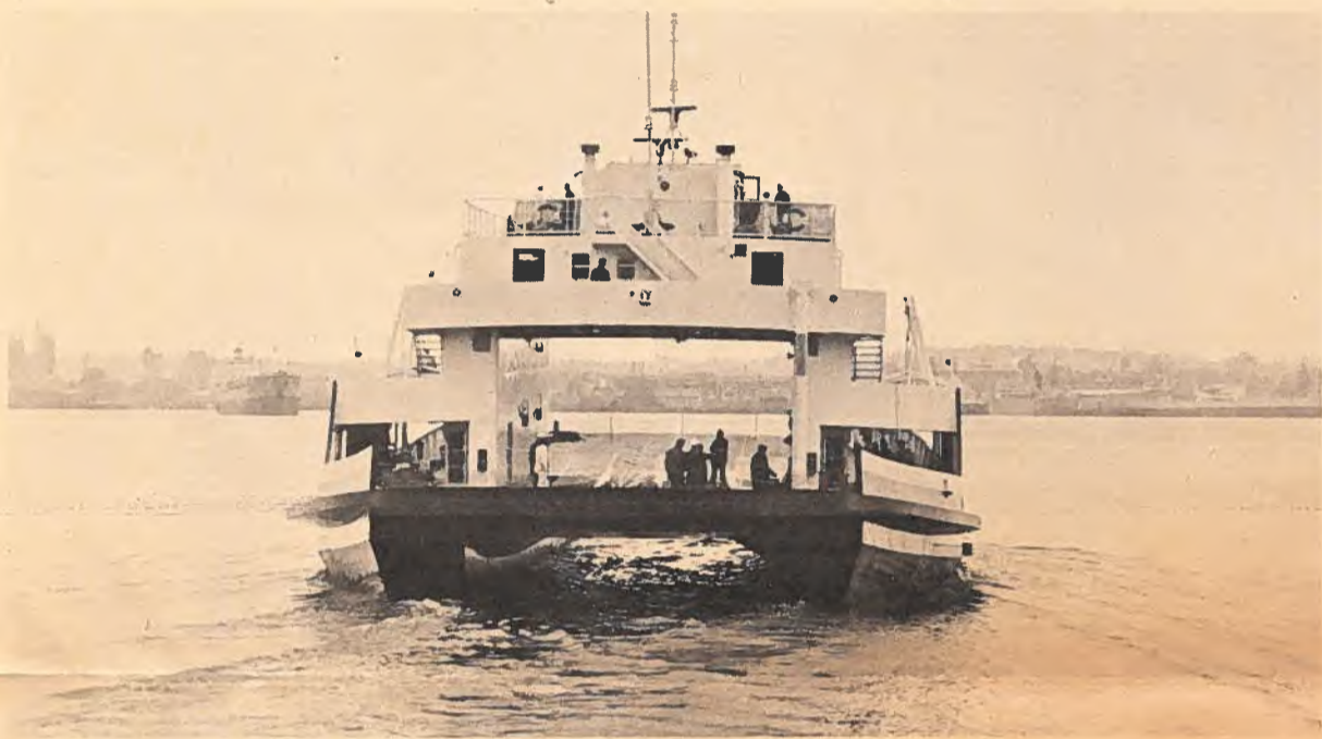
New catamaran hull design developed by Case Existological Laboratories more than doubled this ferry's capacity when she was re-built.
