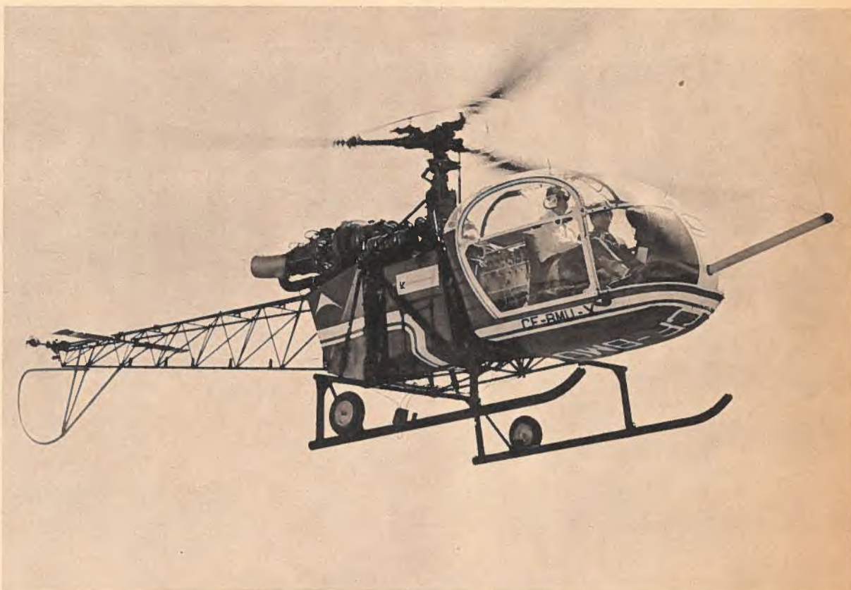
Barringer multi-sensor exploration helicopter, with radiophase; E-phase; air trace (mercury); Gamma-ray spectrometer; electromagnetometer; magnetometer.
