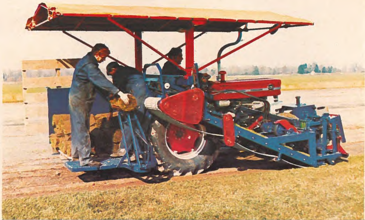
Brouwer's harvester does it all — cuts, rolls and loads up to 1,300 square yards (1,086m 2 ) of sod in an hour.
