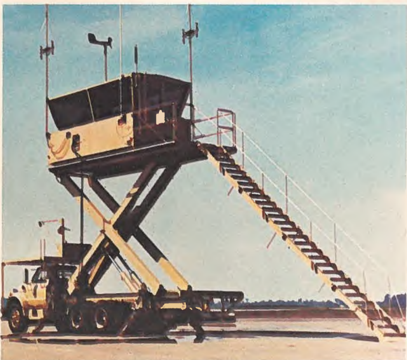
Canadian-designed and produced portable air traffic control tower.
