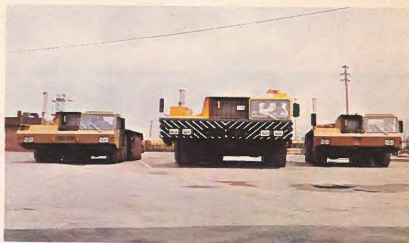
Three of Consolidated Dynamics transit crane chassis. Left to right, model 12615 (total weight lifting capacity 150 tons), 12625 (250 tons), and 10665 (65 tons).
