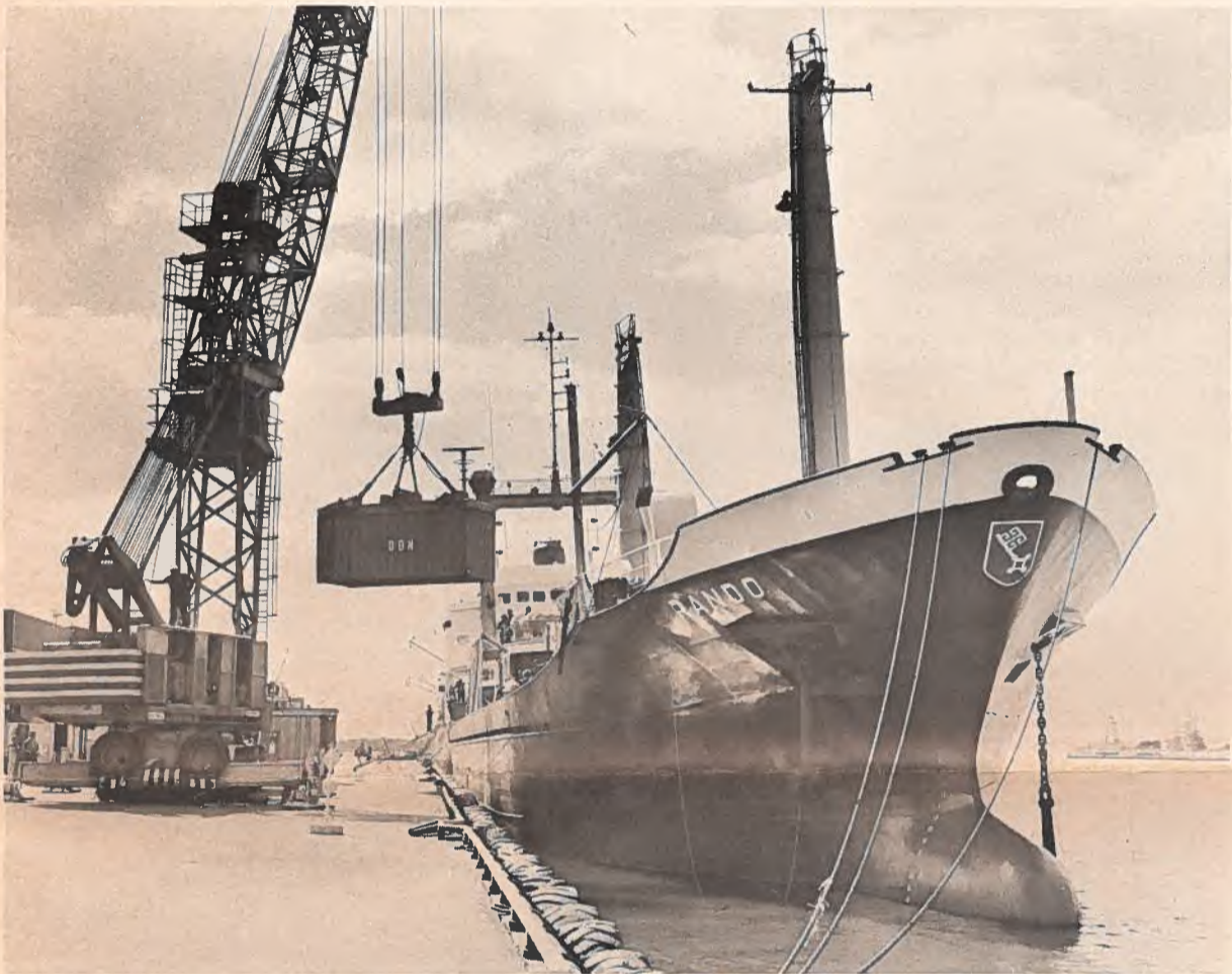
A Gottwald mobile container crane discharges a container from the m/v RANDO, on charter to the Head Line. The RANDO was the first fully-cellular vessel to call at Toronto.
