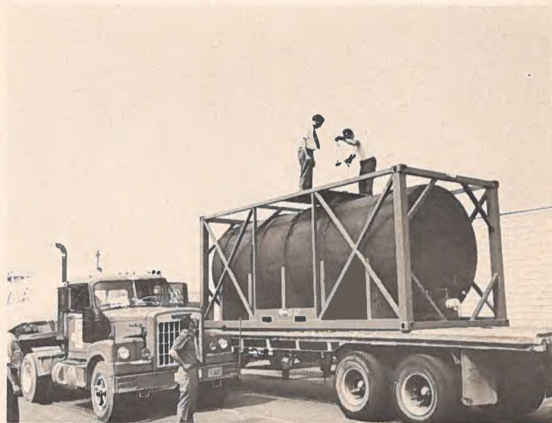
A steel framework in standard container configuration allows this 4,000 gallon (18,200 litre) tank to be handled in the same fashion as ordinary containers. The tank and framework were developed by Steadman Containers Limited and Robin Hood Multifoods for shipment of animal feed ingredients.
