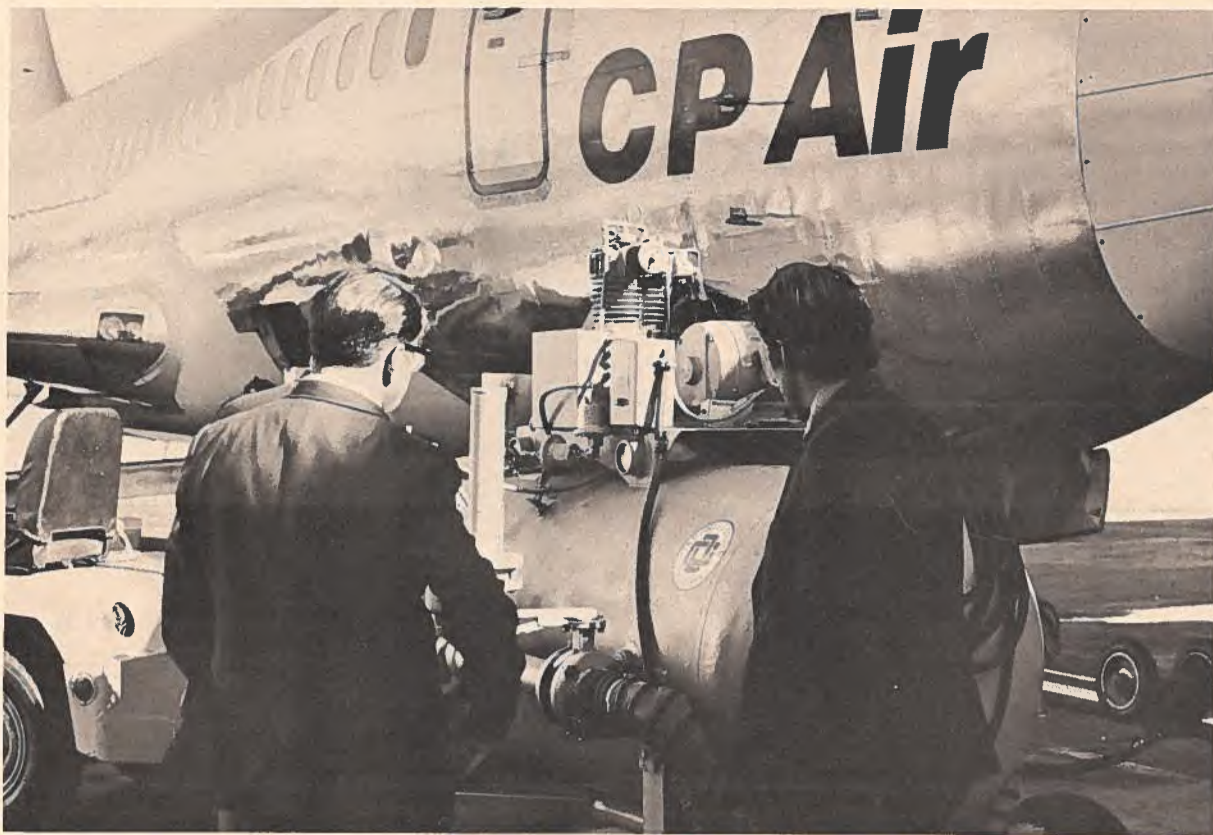
Singer Valve Model 350 Mobile Pneumatic Unit is in use by CP Air and other major airlines.
