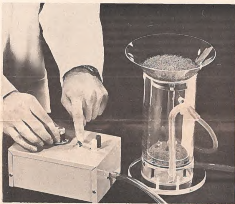
Physico-Medical Systems' Uroflometer has unique ability to measure rate, pattern, time and amount of urine flow.
