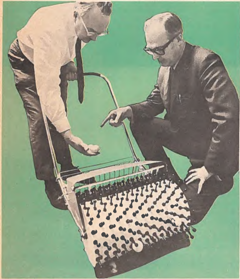
Designer Bill Gamblin (left) with Gord Hovey, president of Hovey & Associates, manufacturers of the Shagmaster. They're discussing the Shagmaster hand-operated golf ball picker. Various multiple units for power towing or pushing are also available.
