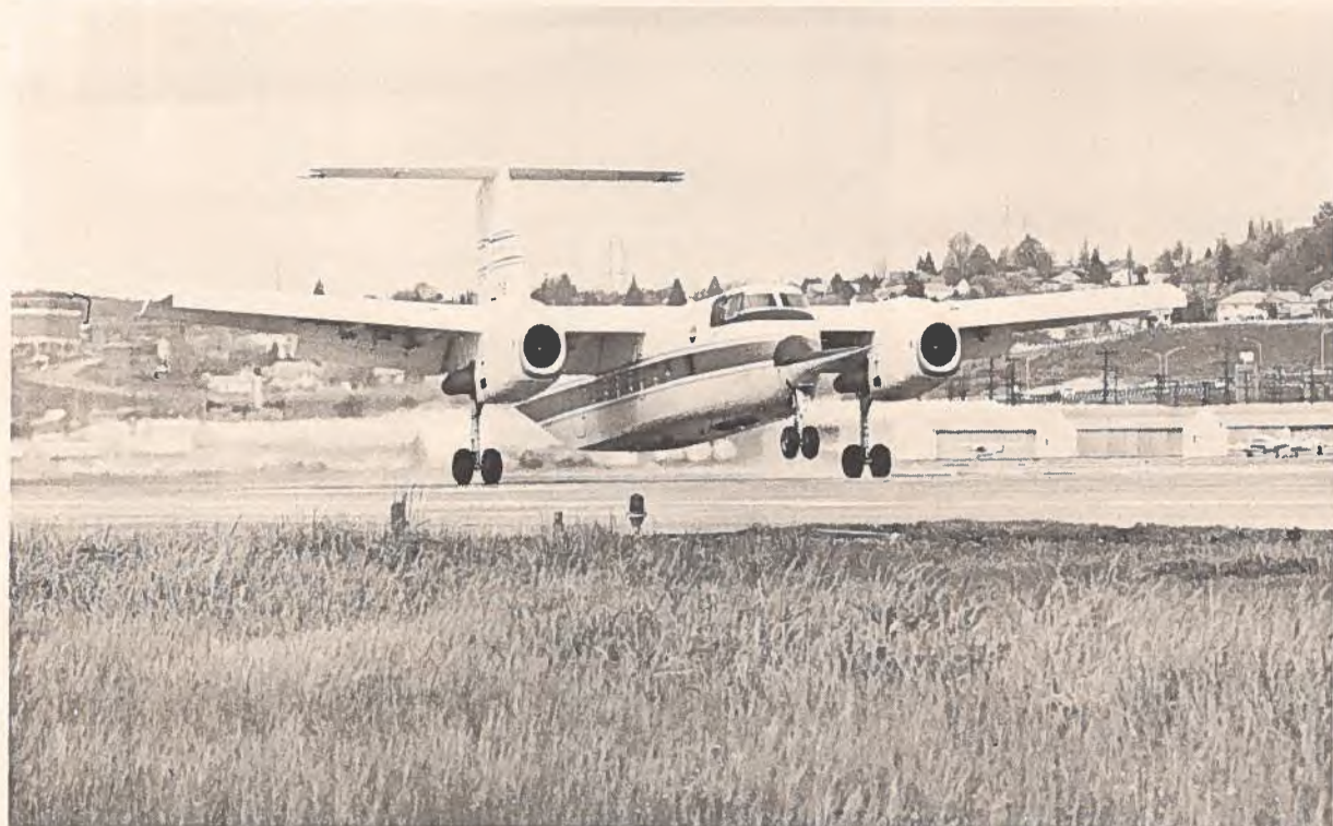
The Boeing/de Havilland "Augmentor Wing" STOL research vehicle flew for the first time May 1, 1972, in Seattle, Washington. The aircraft is a modified de Havilland Buffalo. It is powered by two Spey jet engines specially modified by Rolls-Royce Canada. The experimental aircraft is pioneering a generation of jet-STOL aircraft for the 1980's.
