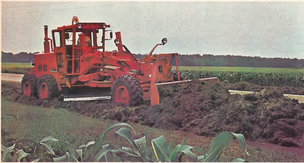
Dominion Road Machinery Co.'s Champion heavy-duty motor grader moves large volumes of dirt with front-mounted bulldozer attachment.
