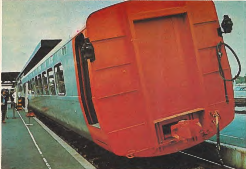
This train is tipsy? No, just tilted — so it won't lurch going round a curve. Light, swift LRC is a product of Alcan-Dofasco-MLW consortium.
