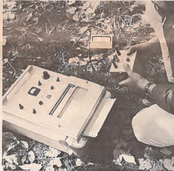
Portable engineering facsimile seismograph, for use with hammer or explosive, produced by Huntex Limited of Toronto.
