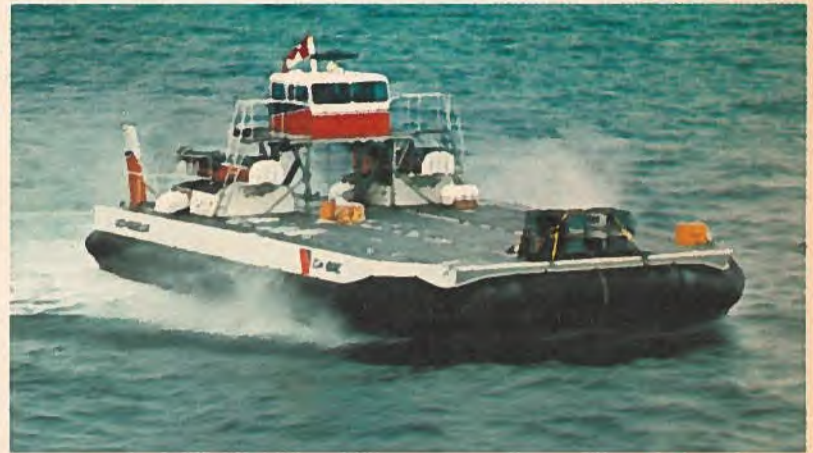
First prototype of Canada's Voyager Heavy Haul Air Cushion Vehicle successfully completed over-water tests at Toronto's Island Airport. These followed one month of winter overland tests in Ontario. Produced by the Grand Bend (Ontario) facility of Bell Aerospace Canada Division of Textron Canada Ltd., it is designed for a project per-ton-mile operating cost one-fourth that of heavy-lift helicopters and is built with prefabricated modules for easy deployment by road, rail or air. Top speed is 50mph (80kmph). Basic flatbed design allows a variety of operational uses.
