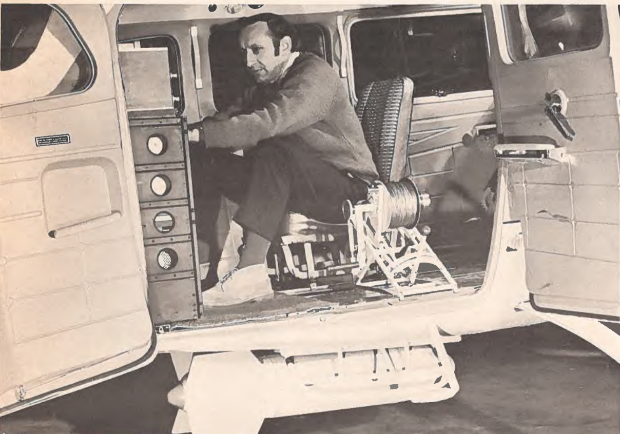
"Torpedo" below plane is receiver for F-400 electromagnetic airborne system, designed and made by McPhar Geophysics Limited. Operator runs four geophysical systems.
