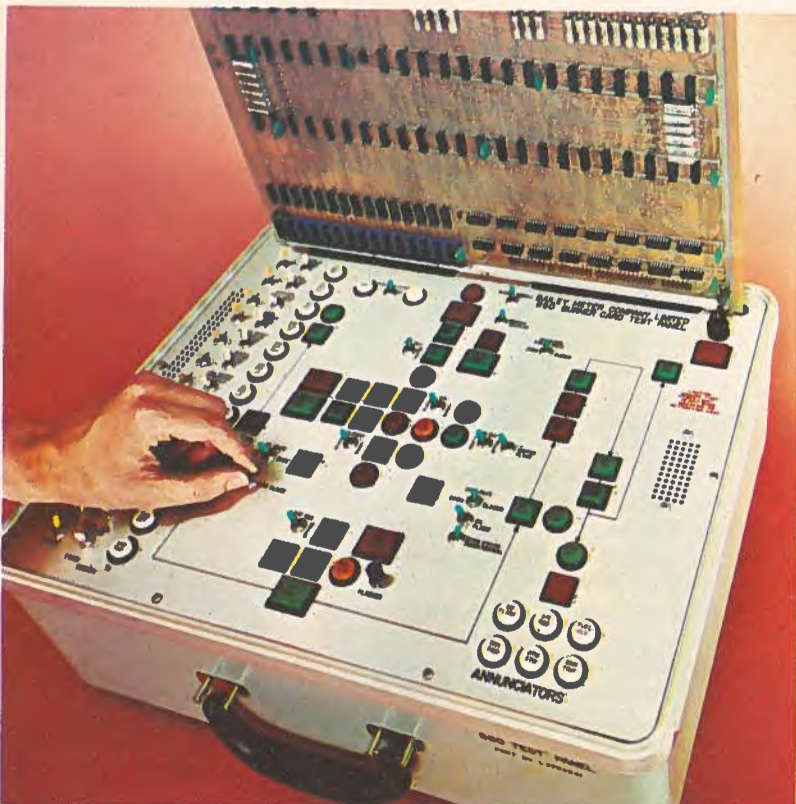
Suitcase-type optional test kit allows in-plant testing of burner logic circuit cards of the Bailey 860 system. The portable kit is complete with power supplies, lights and switches.
