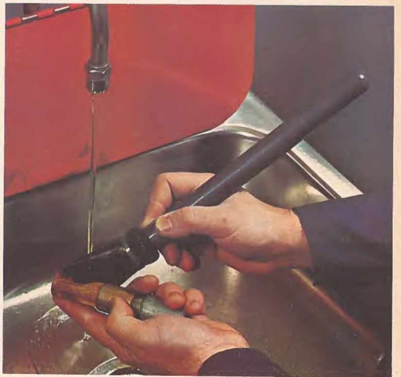
Solv-X Washmaster, the recycling parts washing machine, leaves both hands free for the cleaning job. Solv-X showed its Washmaster at Auto-mechanika '72 in Frankfurt, Germany.
