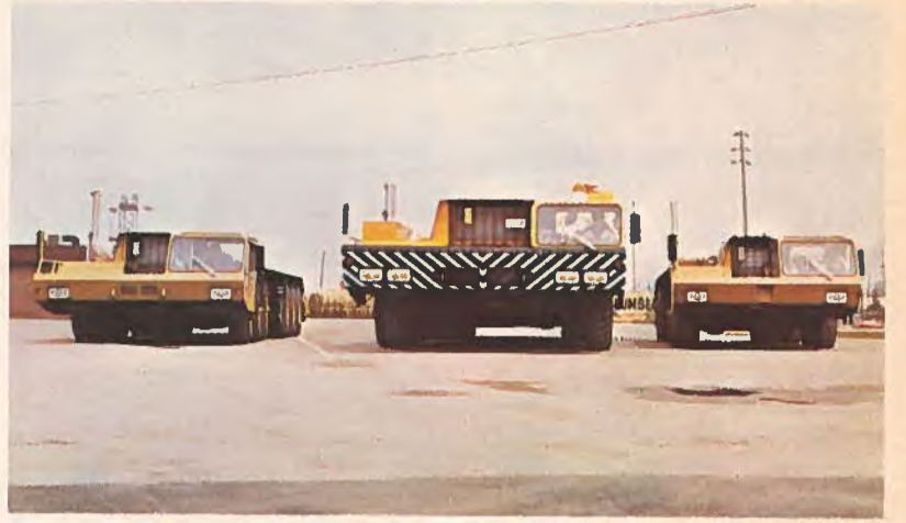
Three of Consolidated Dynamics transit crane chassis. Left to right, model 12615 (total weight lifting capacity 150 tons), 12625 (250 tons), and 10665 (65 tons).
