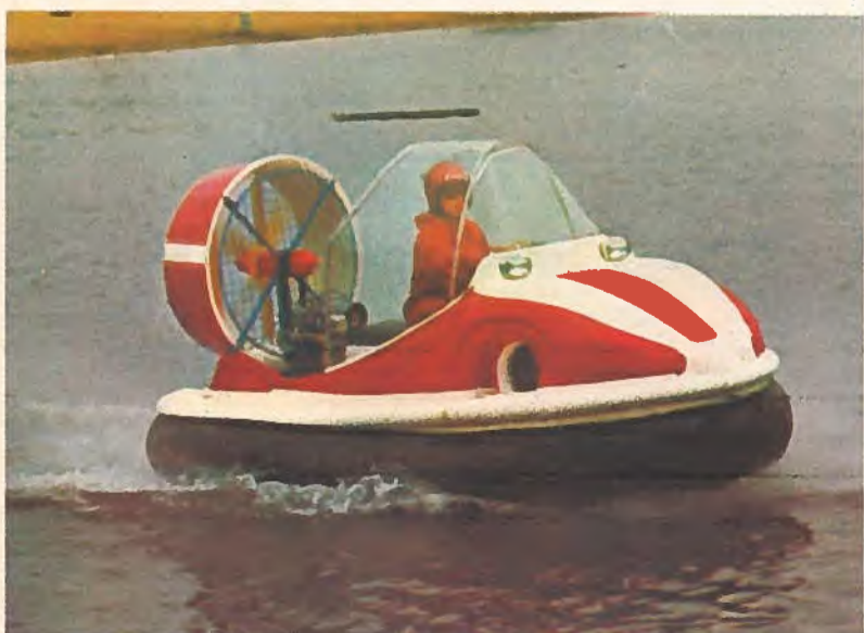
Anticipating that the next boom in the recreational market will involve air-cushion vehicles, MHV Industries Ltd., Ottawa, has produced the Spectra II, which travels from 35 to 65 mph (56 to 105 km/hr). The vehicle spins, hovers on one spot, can change direction instantly.
