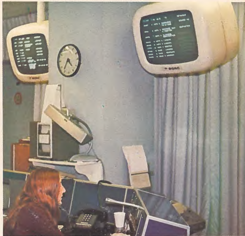
An operator feeds input into the keyboard to display flight arrival and departure information on the television monitors. The DIVCON DG4 flight information television display system, consisting of three basic modular components, is produced by RCA Limited, Montreal, Quebec.
