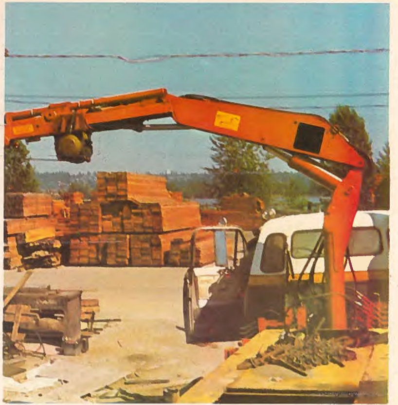
B. C. Gearworks' new Pull Master GT-50 winch — a small horsepower, planetary, hydraulic winch — can be mounted on cranes, tow trucks, drilling rigs, small tug boats and many other pieces of equipment.
