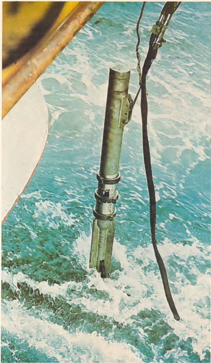
A sonar buoy, used extensively by Kenting Exploration Services Limited, is deployed here to record seismic refraction impulses in Hudson Bay. The unit is a telemetry device which automatically lowers a hydrophone into the water, raises its antenna, receives seismic signals and transmits the information to a receiver on board the survey ship. Kenting is particularly known for its technical skill in conducting marine seismic surveys in the Canadian Arctic. Code 4-1
