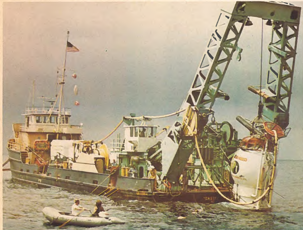
Lockheed service vessel M. V. Coastal Cruiser launches a utility capsule to a subsea oil well in the Gulf of Mexico. The design of the capsule minimizes the cost to water depth ratio and opens up the possibility of economical exploitation of the continental shelves. Lockheed Petroleum Services Limited has also built and successfully tested a manned atmospheric subsea system for producing and servicing oil wells at depths exceeding 1,000 feet (305m). Code 5-2
