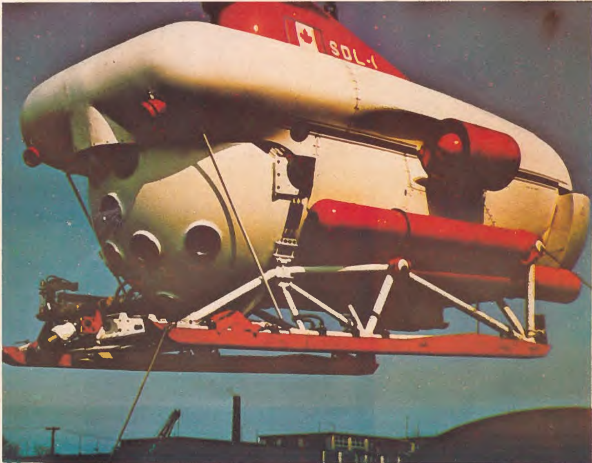
The SDL-1 submersible diver lock-out is designed and manufactured by International Hydrodynamics Company Limited (HYCO). Capable of reaching a depth of 2,000 feet (609.6m), the SDL-1 offers unprecedented flexibility for a wide variety of commercial, scientific and military uses. HYCO is known internationally for its ability to design, build, manufacture and operate submersibles, their tools and support facilities. Code 4-3
