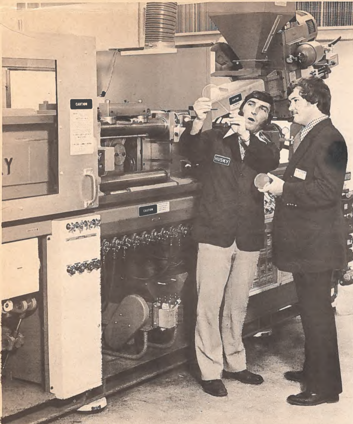
Customer approves a mold and part in Husky's new testroom. Here all molds are tested for two hours before being shipped to customers.
