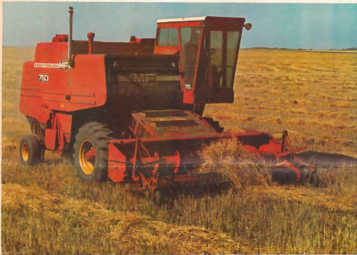
Double flexing nylon tines designed to protect grain heads from breakage or damage are a special feature of this pick-up attachment manufactured by Renn-Cupit Industries Limited.
