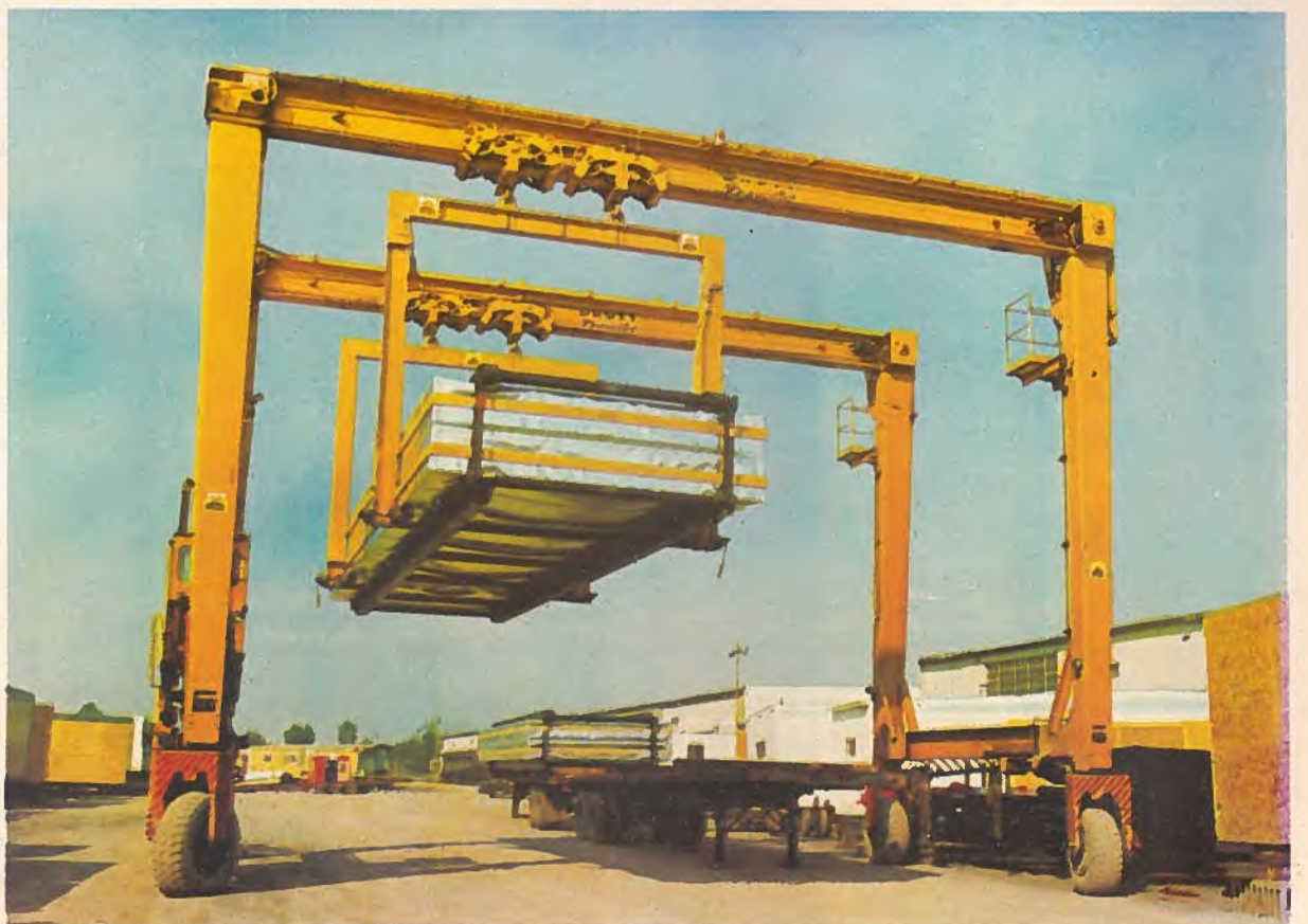
A portable classroom, knocked-down to a height of only 30 inches (762mm) for shipping, is really 9 feet (2.7m) high, 12 feet (3.6m) wide and 37 feet (11.2m) long when assembled. The units are manufactured by Atco (Quebec) Limited and exported internationally.
