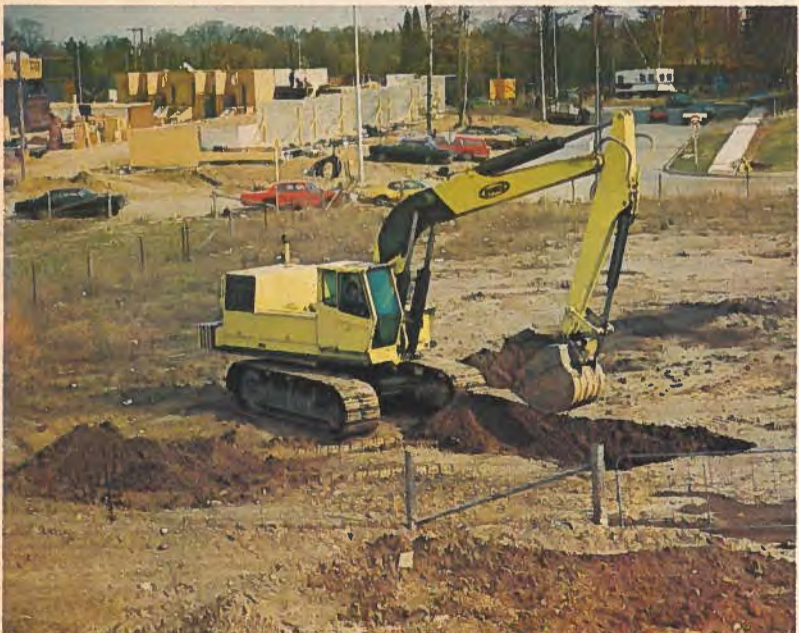
Newest addition to a well known line of hydraulic backhoe excavators is the 6000TT manufactured by Hy-Hoe Corporation Limited, Arnprior, Ontario. With a precision continuous swing at 4.0 rpm, the 6000TT weighs approximately 81,000 pounds (36,774kg) and has a maximum reach — at grade level — of 37 feet, 5 inches (11.3m).
