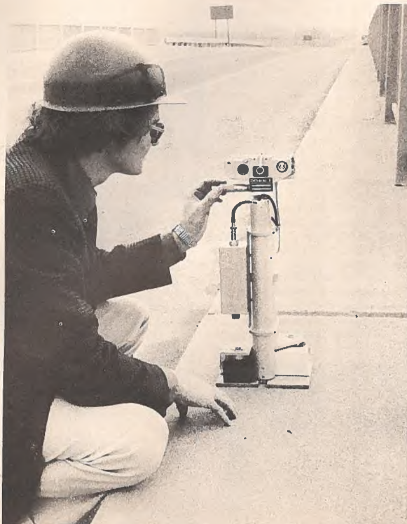
The strain gage, used to measure expansion in such structures as bridges, tunnels and concrete buildings, can be permanently installed in the structure and read anytime in the future with the same accuracy as the day of installation.
