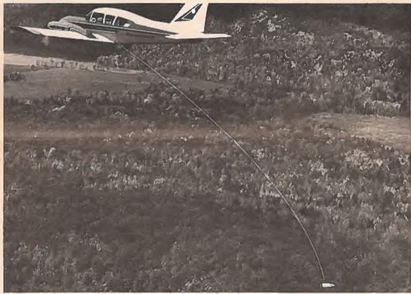
A Kenting Earth Sciences (formerly Spartan Aero Limited) airplane trails an airborne magnetometer or "bird" for mineral exploration over the Canadian Shield. The company provides resource exploration and development services on an international scale.
