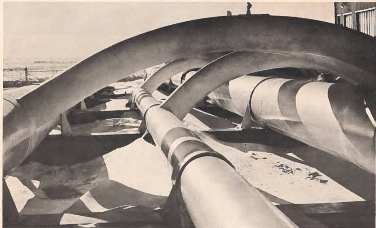
Steel-Flo's drawn outlet headers are the first made in Canada for the oil and gas transmission lines and the petrochemical and nuclear industries.
