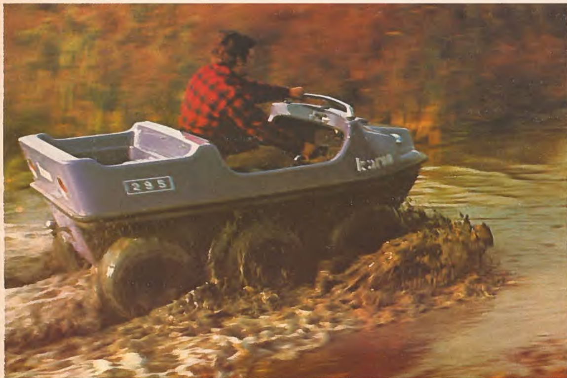
Karou does it all — climbs 45-degree hills, pulls twice its own weight, churns its way through mud, water and snow, and turns on a dime. This all-terrain vehicle is manufactured by Karou Incorporated, Drummondville, Quebec.
