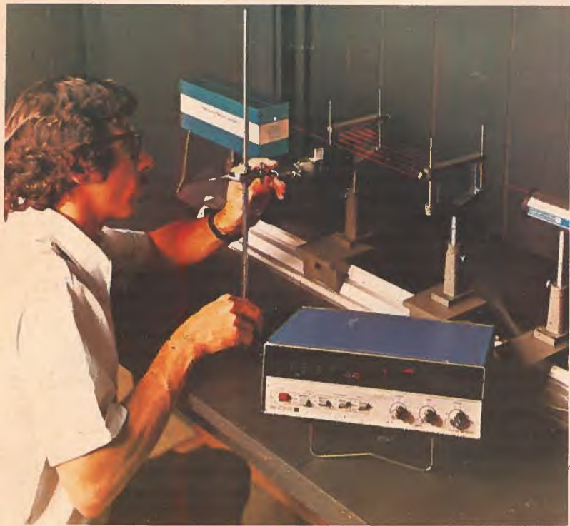
High resolution spectral absorption measurements are made with Alpha-metrics' Model DC1010 radiometer/photometer. The laser beam is reflected ten times between a pair of mirrors before landing on the radiation detector. This procedure increases the measurement sensitivity by ten times and results in a more precise determination of spectral absorption. Here, an operator inserts a filter glass for measurement.
