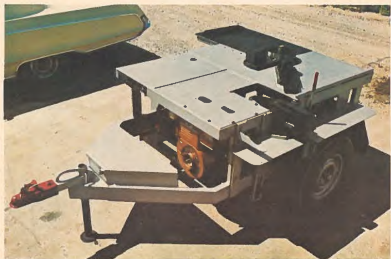
The Journeyman Bender by Hydrex Industries Limited bends or shears reinforcing rod and is available in metric or imperial systems.
