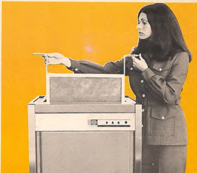
Operator inserts basket in automatic color paper processor designed and manufactured by Braunoehler Company.
