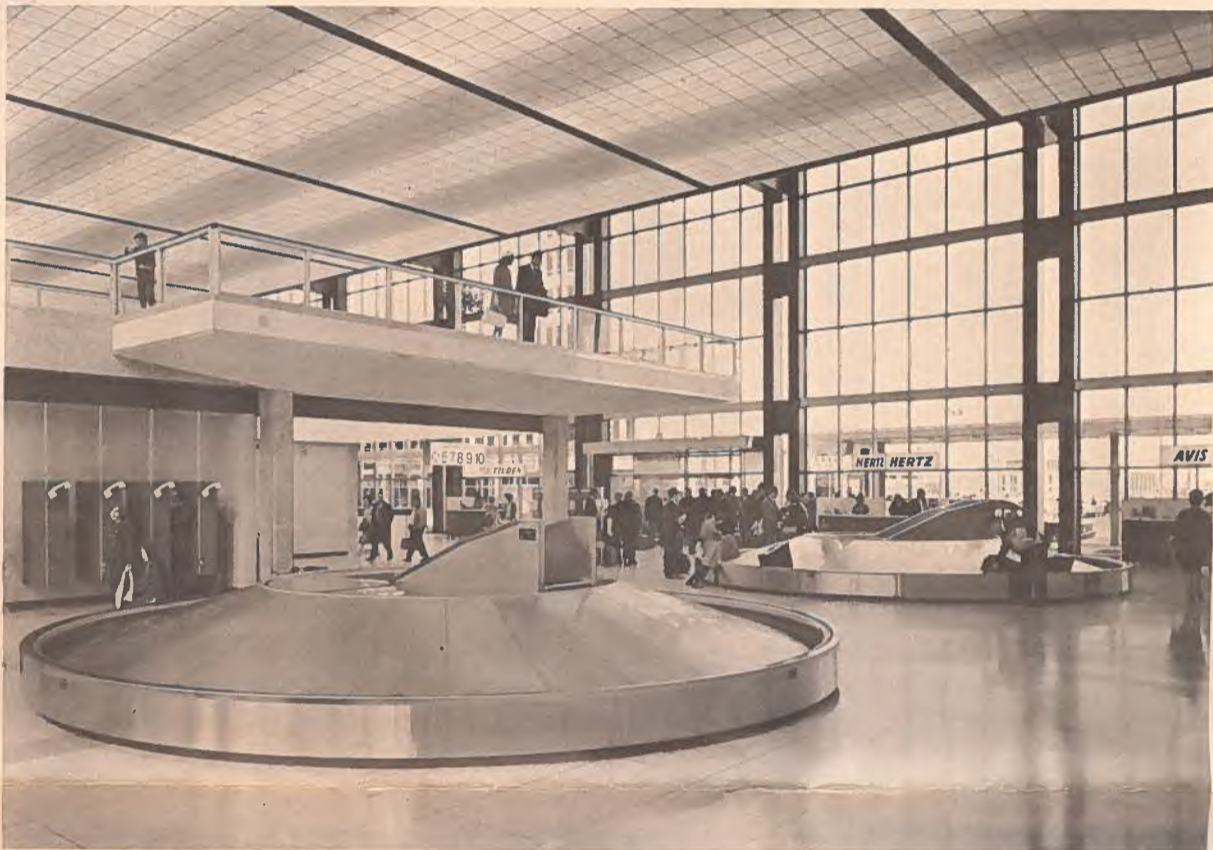
A first — the Carrousel luggage dispenser originally designed by Mathews, was the first dynamic system which permitted passengers to remain stationary and the luggage to be delivered to their position. Over 200 such units are now used in air terminals throughout the world.
