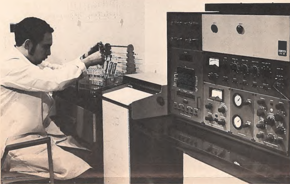
Scientist at T. W. Beak Consultants laboratory uses a gas liquid chromatograph to measure the level of organic compounds in industrial waste water.
