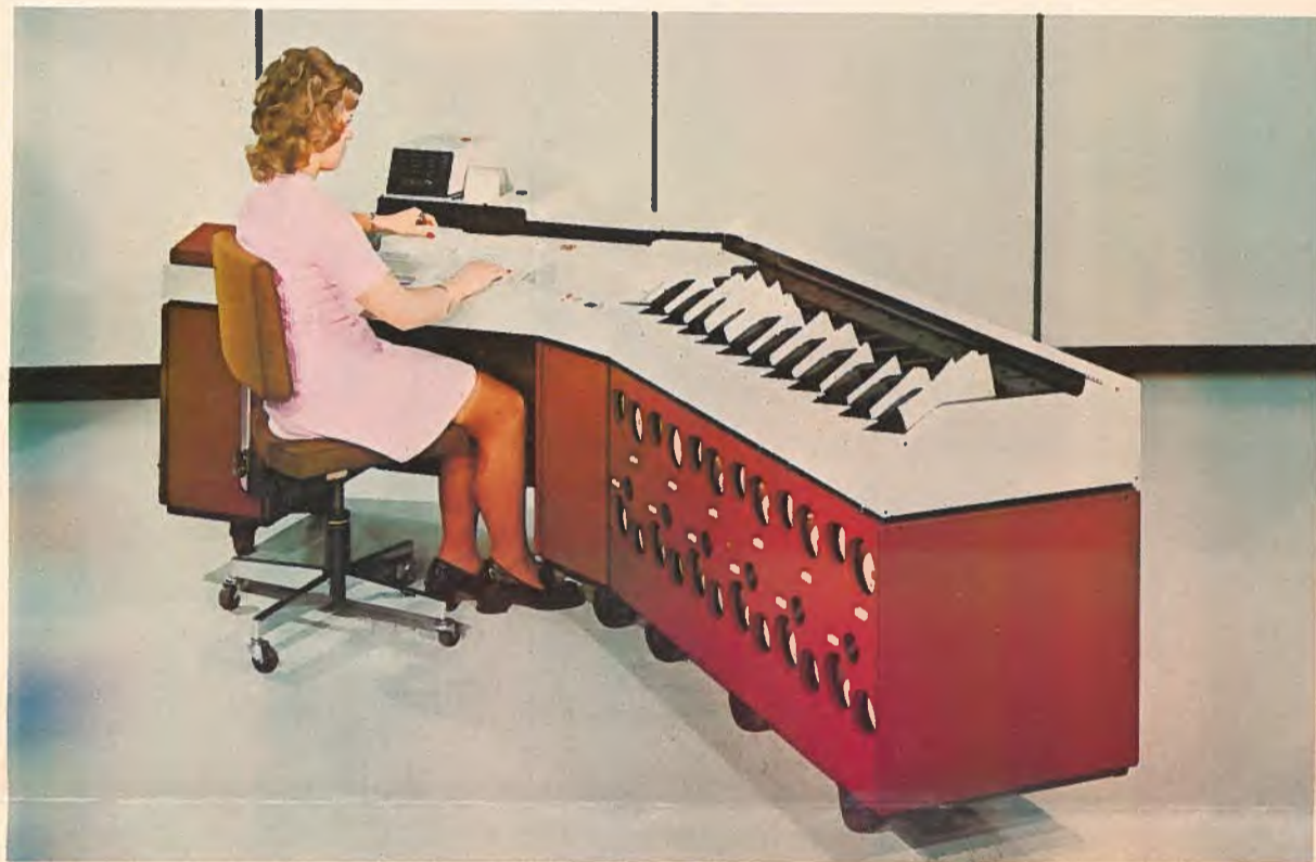
Operator works at NCR Canada's new 775 system for proofing and encoding bank documents. The system is quicker and more flexible than previous equipment.
