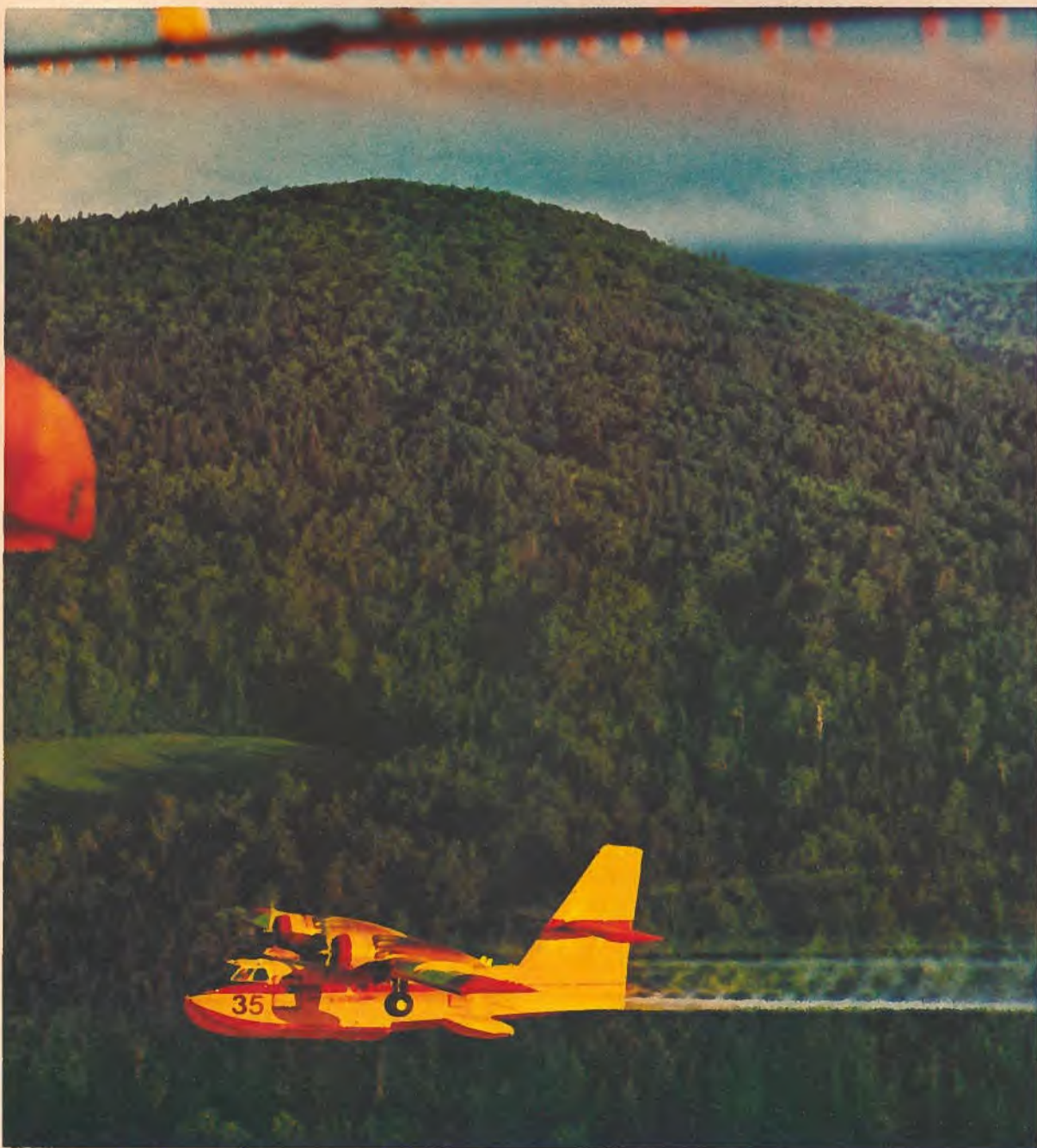
The CL-215 amphibian aircraft has been used to spray spruce forests against budworm infestations. The plane is also a "water bomber" for fighting forest fires and is used for aerial surveying, patrol, search and rescue operations.
