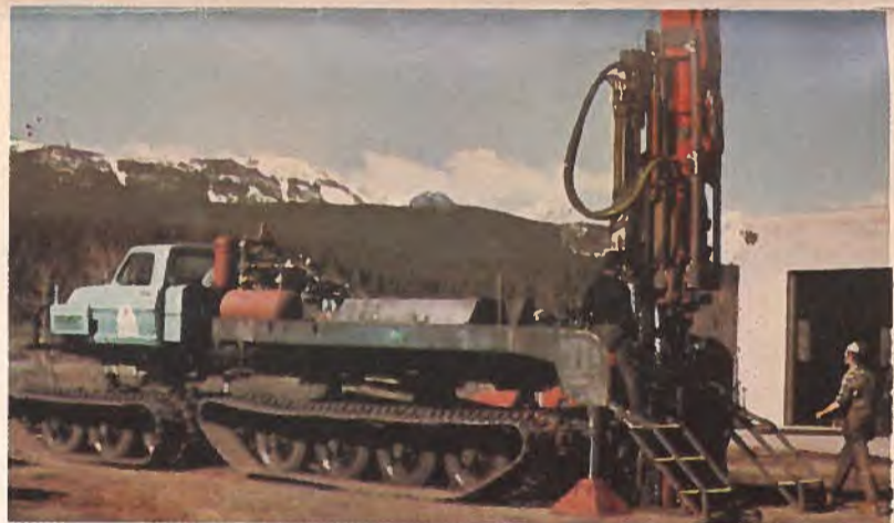
Drills for use in civil construction, soil sampling, mineral exploration, and offshore mineral and soil investigation are manufactured by Drill Systems Inc., a subsidiary of Upper Canada Resources Limited, Calgary, Alberta. The company's Becker hammer drills and Center Sample Rotary (CSR) drills are self-contained drilling units that can be mounted on truck, steel track, soft track carriers or skid frame. Code 2-4
