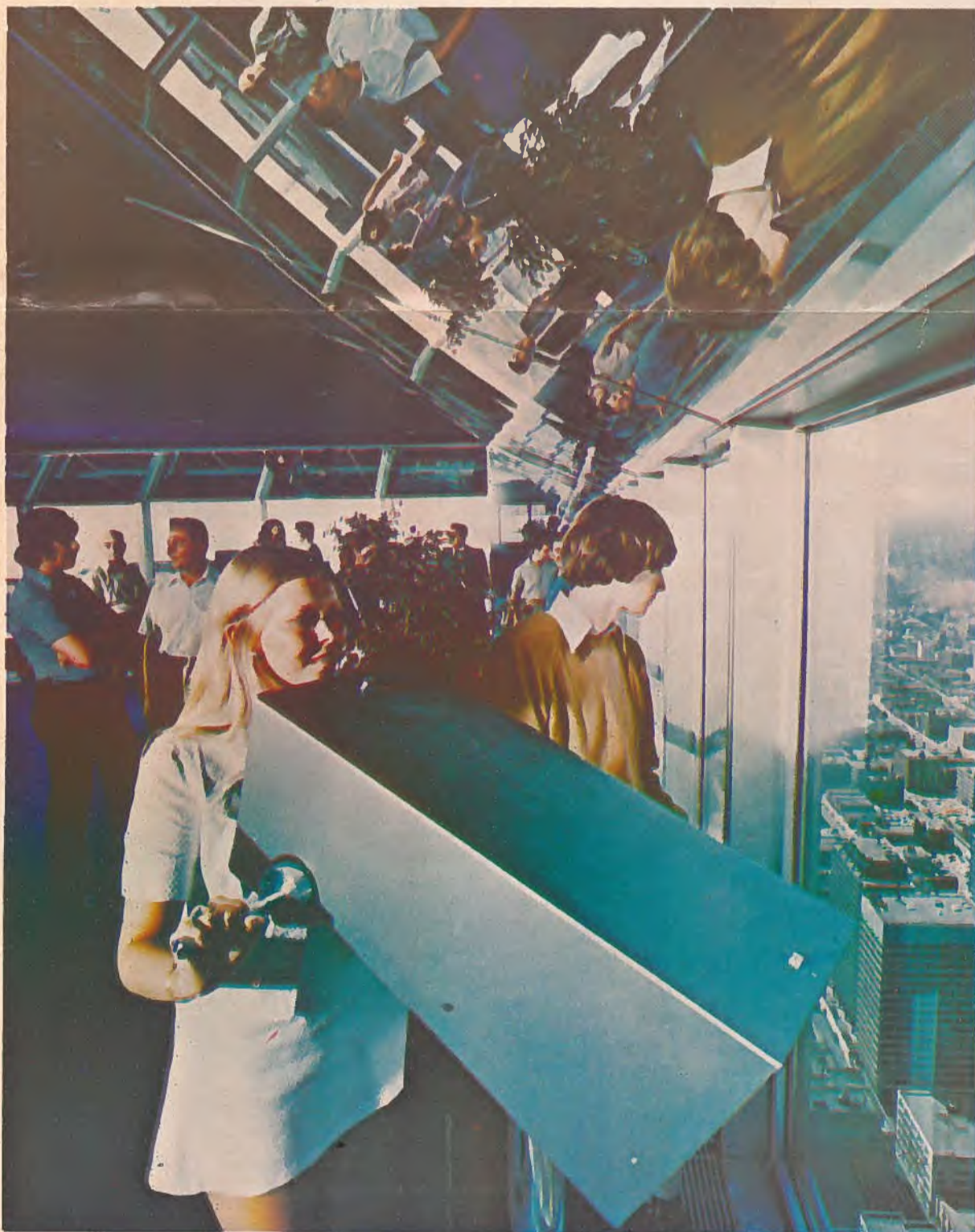
From the 57th floor an observer views the City of Toronto through this 30 magnification observation gallery telescope designed by Bredberg Optical & Scientific of Markham, Ontario. The styling, optical system and user-adjustable height lever make it one of the world's most advanced observation gallery telescopes. Two separate optical trains, one for each eye, preserve the three dimensional aspect of normal vision — even at night when it is possible to decipher car license plate numbers a mile (1.61km) or more away. The telescope also features a mechanism which yields — in only two seconds — a focus range of from 110 feet (33.5m) to infinity. The highly reliable unit can be re-styled to meet the need of practically any observation gallery. For instance, the Bredberg telescopes to be used in the John Hancock Building in Boston, Massachusetts, will be of circular shape to match the building's decor. And they will be suspended from the ceiling to reduce installation costs and provide additional column-free floor space. Bredberg Optical & Scientific, whose forte is telescopes, optics and specialty systems, is also noted for its six and 12-inch (15.2 and 30.4-cm) aperture Reflector telescopes for the hobby and school market. Code 7-2
