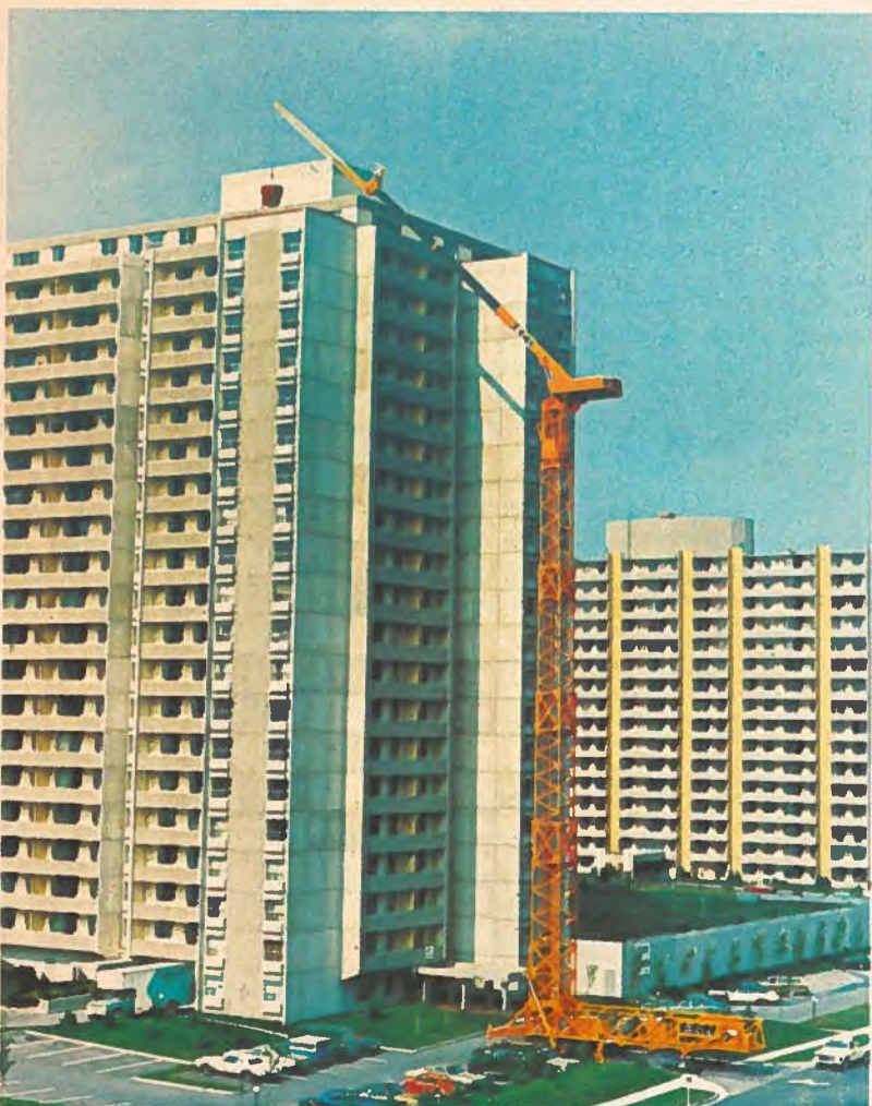
Unique, versatile and speedy — that's the GCI 5400, a completely mobile self-erecting hydraulic crane manufactured by General Crane Industries, London, Ontario. At its maximum height of 255 feet (77.7m), the crane can reach out 115 feet (35.1m). It can be set up as close as nine feet (2.7m) to the side of a building and can travel at a highway speed of 50mph (80.5km/hr).
