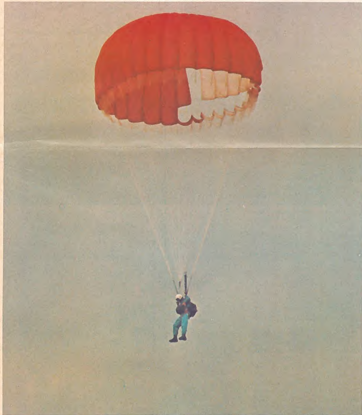
On a slow, safe descent, this jumper is wearing the new TU 7 Gore Search and Rescue Canopy (SAR) from Irvin Industries Limited, Fort Erie, Ontario. Canopy deployment malfunctions are eliminated with the SAR chute because of Irvin's special net skirt. Code 7-232
