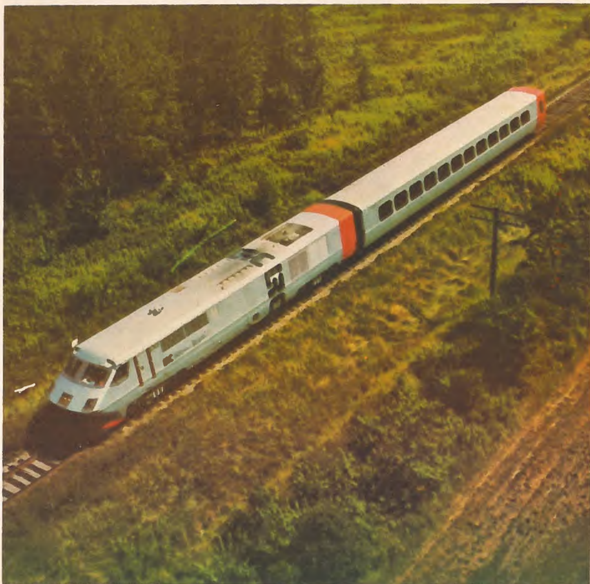
Canada's latest innovation in intercity passenger rail travel, the LRC (light, rapid, comfortable) locomotive and coach undergoing a test run between Montreal and Ottawa. With a continuous terminal-to-terminal speed of 100mph (161km/hr), the diesel electric locomotive and 84-passenger coach is attracting interest around the world.
