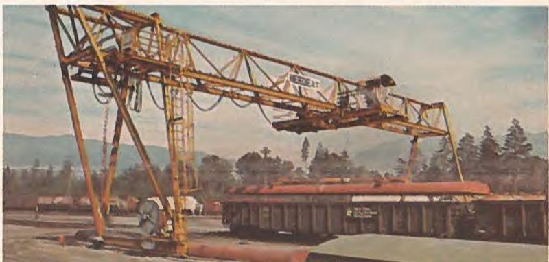
One of North America's original manufacturers of climbing cranes, Heede International Ltd. constructs cranes in capacities and sizes from those with a 100-foot (30.5-m) jib and 6,000-pound (2,724-kg) capacity to cranes with a 205-foot (62.5-m) jib and a 12,000-pound (5,448-kg) capacity. This "cover-lifter" portal crane was specially designed and built by Heede for Vancouver Wharves of North Vancouver, British Columbia. The crane efficiently removes, temporarily stores and ultimately replaces fiberglass covers which are placed over gondola cars during transportation of concentrates.
