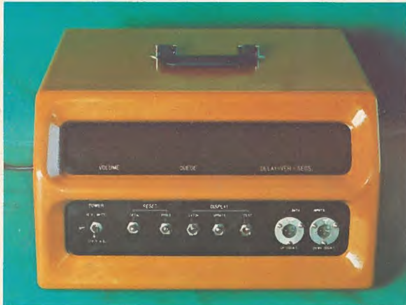
Attractively housed in a streamlined fiberglass case with recessed instrument switches and display, the MPT computer from SDS Technical Devices Ltd. of Winnipeg, Manitoba, gives digital readouts of six types of traffic parameters.
