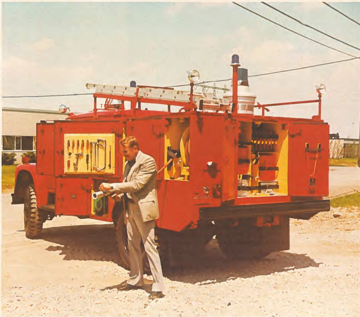
Four fire fighting vehicles, such as this one, were recently purchased by the International Airports Authority of India. They will be used as rapid intervention vehicles to reach an accident site quickly, initiate rescue and provide means of fire protection before the arrival of major units of equipment — a feat easily accomplished since the vehicles can accelerate from 0 to 50mph (0 to 80km/hr) in only 34 seconds and cruise at an average speed of 63mph (100km/hr.). The foam, water or dry chemical carriers are manufactured by C-D-N Research & Development Limited, Mississauga, Ontario.
