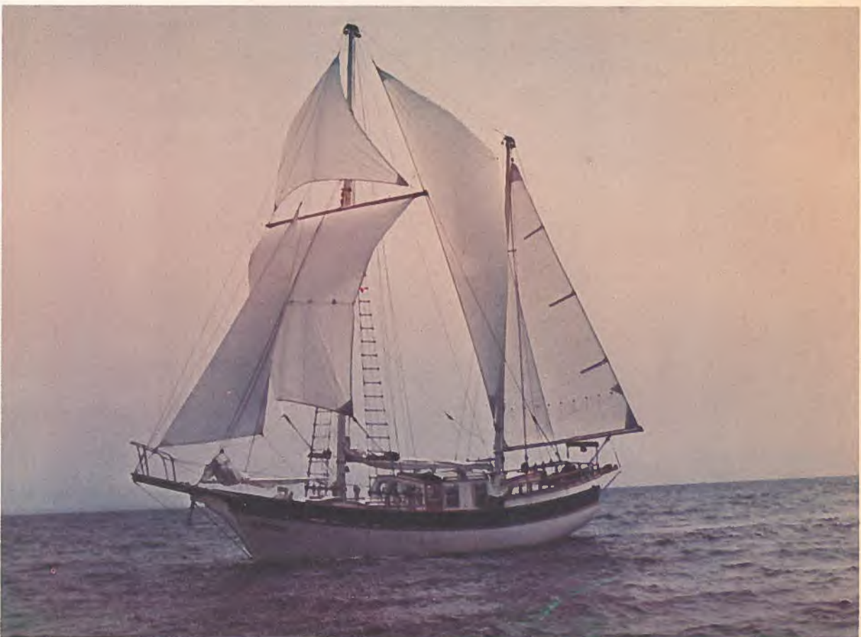
Resplendent in her revolutionary period brig rig — crossing seven yards — the Aquarius brig "Rattlesnake" undergoes power and sailing trials on St. Mary's Bay, Nova Scotia. Built for a Long Island, New York, buyer, this 55-foot (16.7-m) "modern" brig-of-war is complete with swivel guns, freezers and diesel generators.
