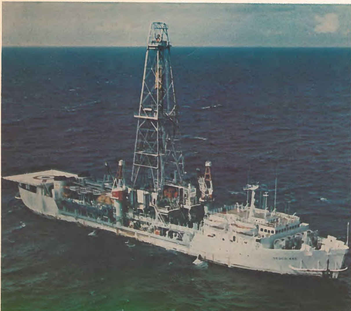
This self-propelled, dynamically positioned drilling ship, the Sedco-445, is manufactured by Halifax Shipyards, a division of Hawker-Siddeley Canada Limited — a company that is known internationally for the construction of its floating oil rigs, the largest of their kind in the world. Also being constructed by Halifax Shipyards is a second drilling ship, the Sedco-471. This ship, with an overall length of 470 feet (143.3m), has three cranes, a 147-foot (44.8-m) derrick and a drilling depth of 20,000 feet (6,096m). With twin screw propulsion and 12 thrusters, the Sedco-471 has a maximum draft of 24½ feet (7.5m). Code 5-350
