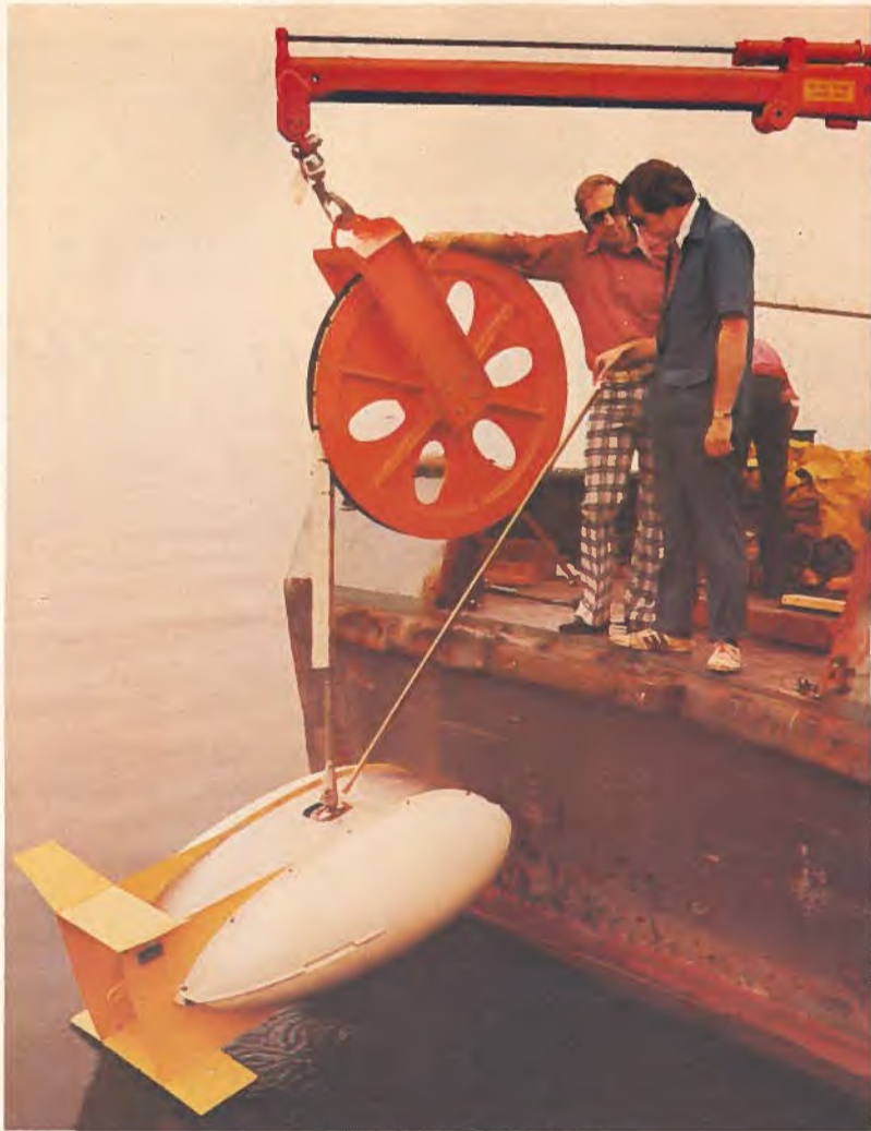
The combined efforts of two Canadian companies have produced this unique underwater system that, compared to previous methods, more effectively gathers data from the ocean bottom. Whereas previous systems were towed on the surface, the newer system — which contains highly sophisticated oceanographic measuring equipment — is towed underwater and records data required to solve ocean engineering problems, such as offshore oil rig replacement, laying pipelines underwater and the design of new port facilities. The companies involved in the joint venture are Fathom Oceanology of Port Credit, Ontario and Hunttec (70) Limited, Toronto, Ontario. The companies are also noted for their submarine antenna towing systems and stationary moored buoys for water data sampling (Fathom); and for the manufacture of components and systems which provide accurate cross sectional profiles of sub-bottom geology of water-covered areas (Hunttec).
