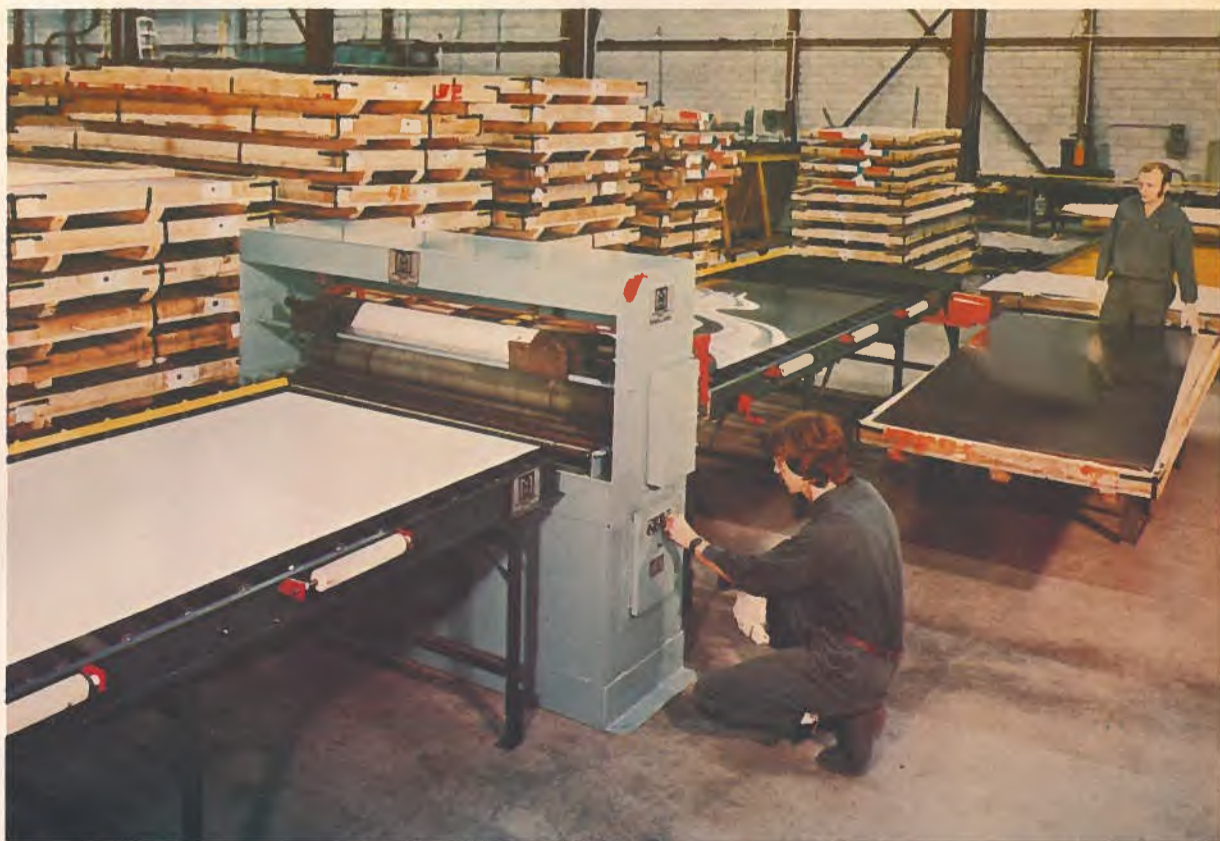
At the touch of a button, the Metalmac tape applicator deposits a wrinkle and bubble-free coating of plastic, vinyl or fabric to sheet materials to protect them during further processing and handling. This Model T4800, will coat sheets up to four feet (1.22m) wide including narrow strip widths, and is adjustable for thicknesses of .016 inches (.04cm) up to 1/4 inch (0.6cm).
