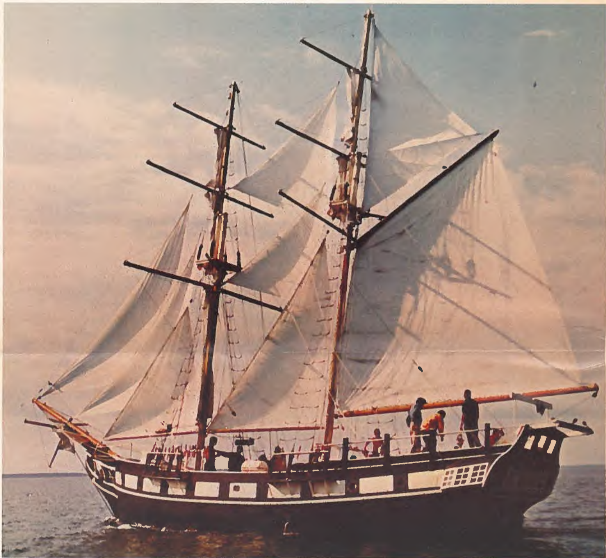
Resplendent in her revolutionary period brig rig — crossing seven yards — the Aquarius brig "Rattlesnake" undergoes power and sailing trials on St. Mary's Bay, Nova Scotia. Built for a Long Island, New York, buyer, this 55-foot (16.7-m) "modern" brig-of-war is complete with swivel guns, freezers and diesel generators.
