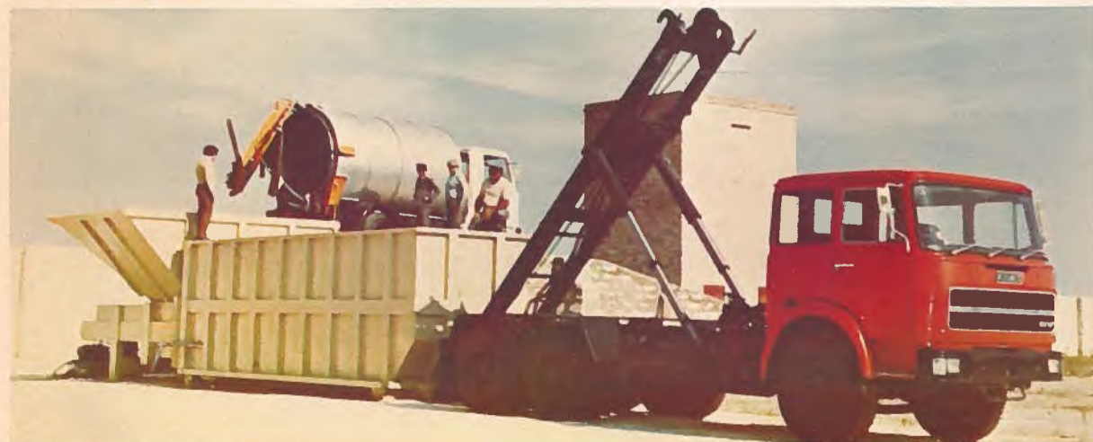
An innovative solid wastes transfer system uses stationary compactor/container and roll-off hoist designed and manufactured by Atlas Hoist & Body Incorporated. One such system is currently being used in the town of Lucera, Italy.
