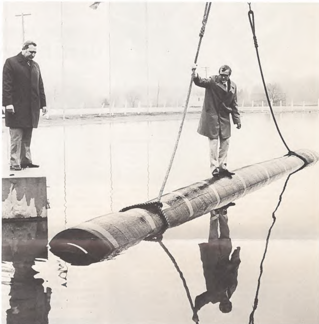
These company representatives conduct a buoyancy check on a section of B. F. Goodrich's new floating oil hose. The hose is designed to deliver oil between off-shore pumping stations and supertankers.
