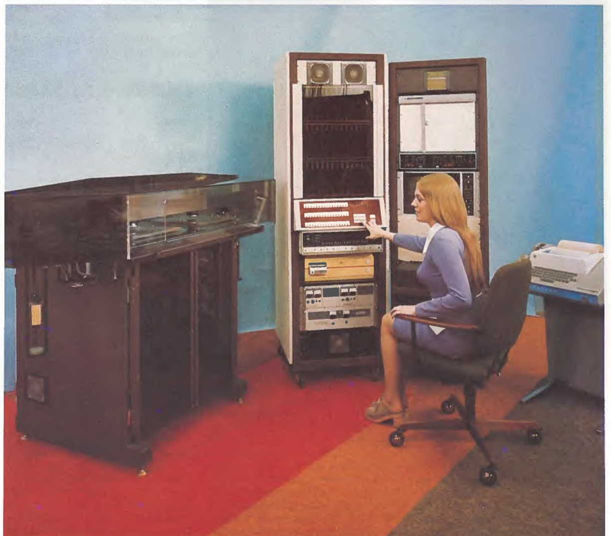
This Photo Mapper is the nerve centre of the sophisticated equipment developed by Gestalt International Limited (formerly Hobrough Limited) of Vancouver, British Columbia. Operator monitors printing process which compensates for displacements in aerial photos. The resulting product is a photo image with conventional map accuracy.
