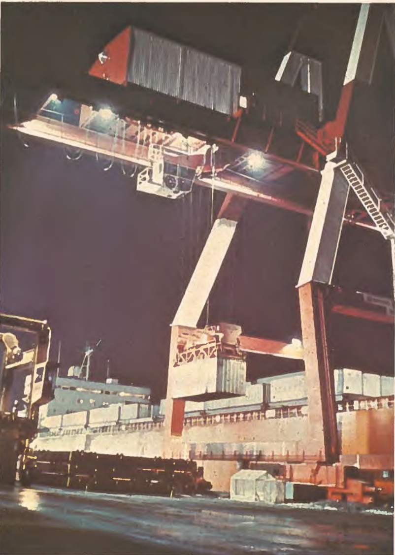
One of the three 45-ton (41-metric ton) gantry cranes of the Halifax container terminus working the night shift.
