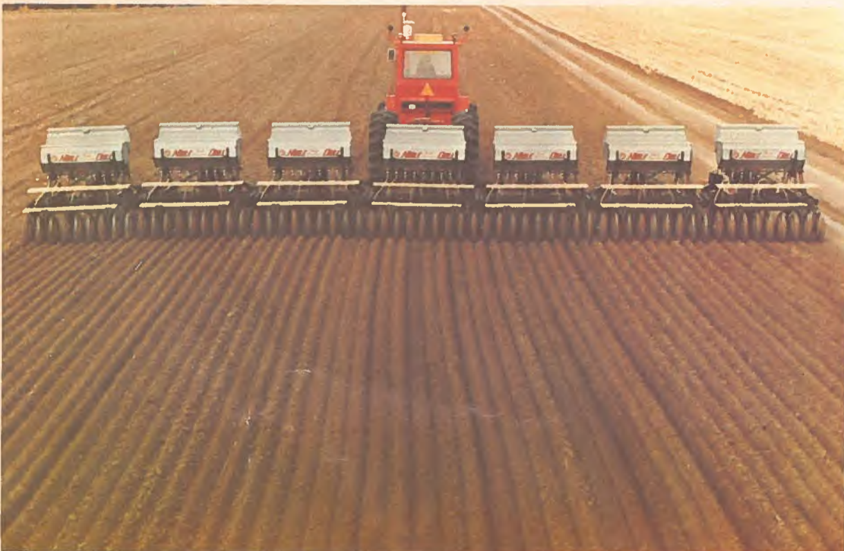
The Noble DK-5 High Clearance Drill seen here in action permits sowing down to firm moist soil without covering seeds to excessive depth. Noble also manufactures three-point cultivators that are ideal for orchards, vineyards, tree belts, row crops and small farms.
