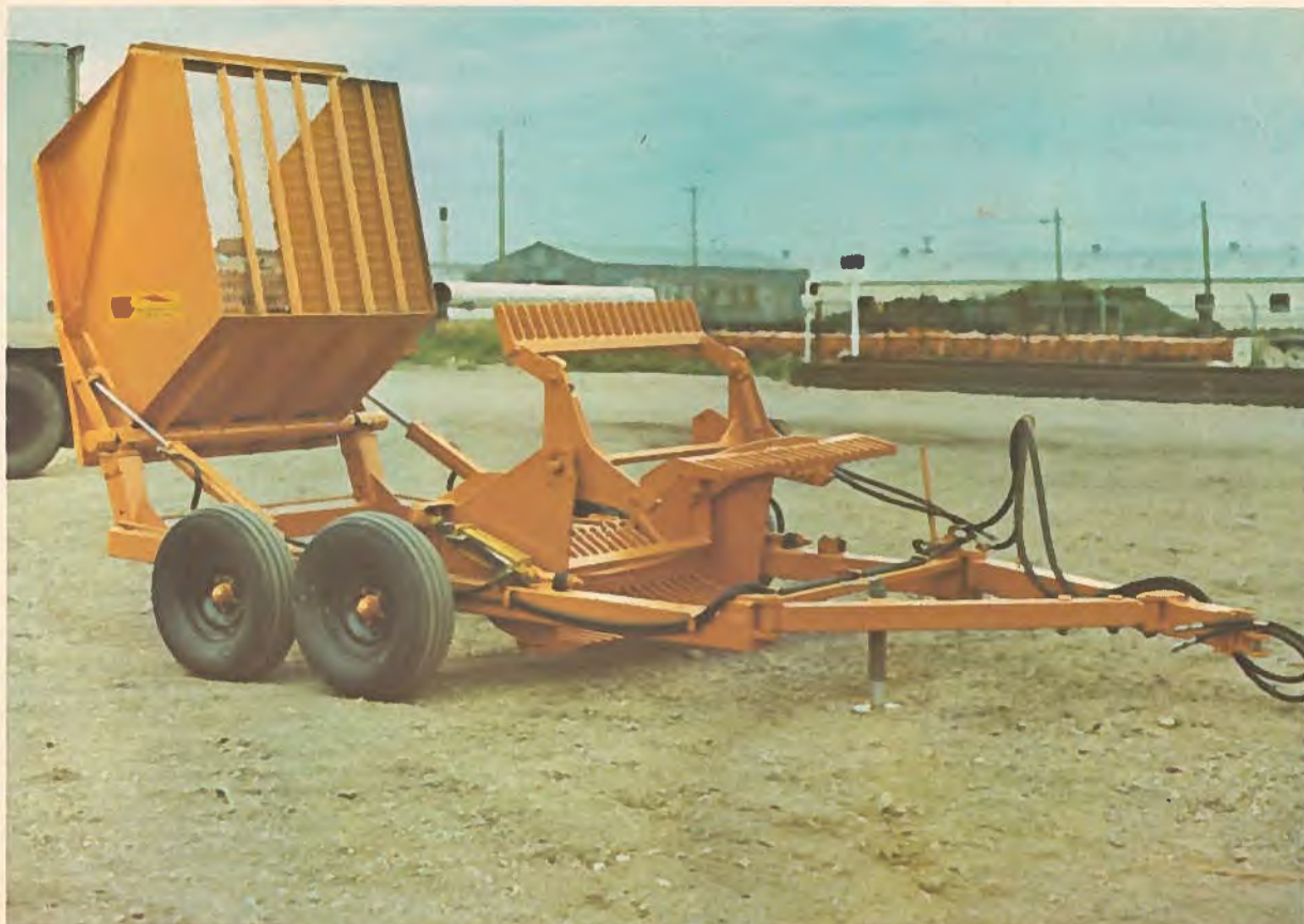
The RR-600 Rotary Rock Picker from Rite Way Mfg. Co. Ltd., is the largest machine of its type on the market. It features an hydraulically-controlled picking height and has a minimum five-ton (4.5-metric ton), three-cubic yard (2-m 3 ) hopper capacity. Its powerful hydraulic motor can be jammed or stalled without damage and it shuts off to pick up larger rocks.
