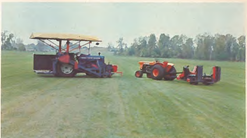
The job of mowing grass or rolling, slabbing and folding sod is a simple task when using machinery manufactured by Brouwer Turf Equipment Limited of Keswick, Ontario. Brouwer's Model A3 sod harvester, shown here with canopy, will roll, slab or single fold turf grasses in 15, 16, 18 and 24-inch (38, 41, 46 and 61-cm) widths of cut. The company's P.T.O. gang mower can mow grass up to 10 inches (25cm) high.
