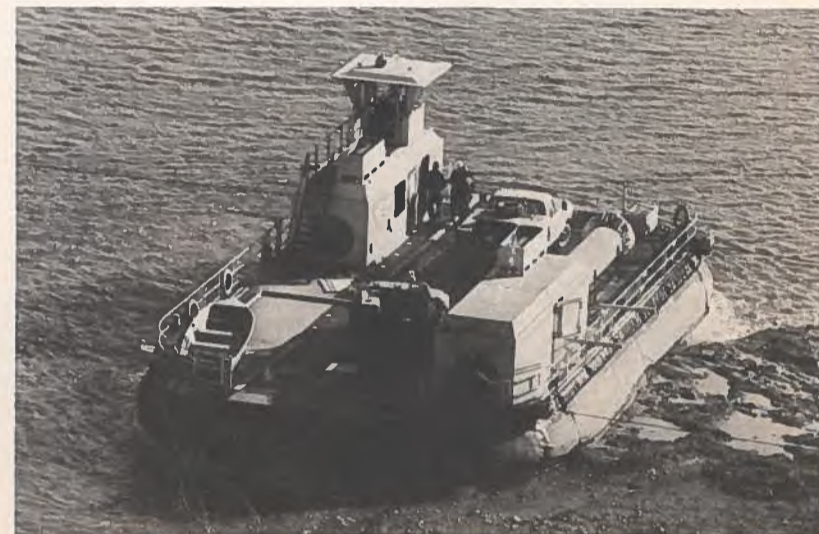
Pioneer I, in service as a hoverferry in Alberta, is 66 feet (20 m) long and 36 feet (11 m) wide. It carries two identical power packs, each of which has a Caterpillar diesel to drive air fans and hydraulic pumps.
