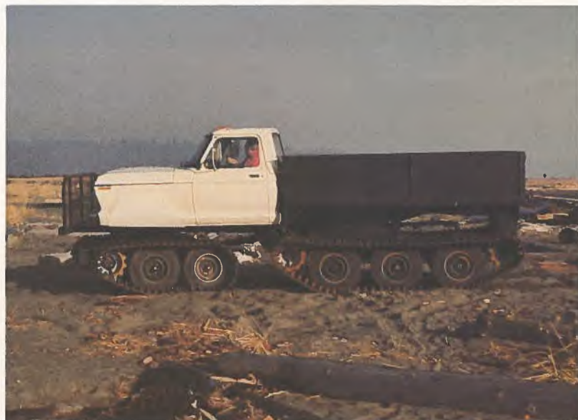
Any ordinary highway vehicle can be quickly converted into an All Terrain Vehicle with Demac Engineering's tracked undercarriage which will get men and materials to remote job sites. Once the job has been completed and the undercarriage is no longer required, it can be easily removed and the vehicle used with tires for more conventional terrain.
