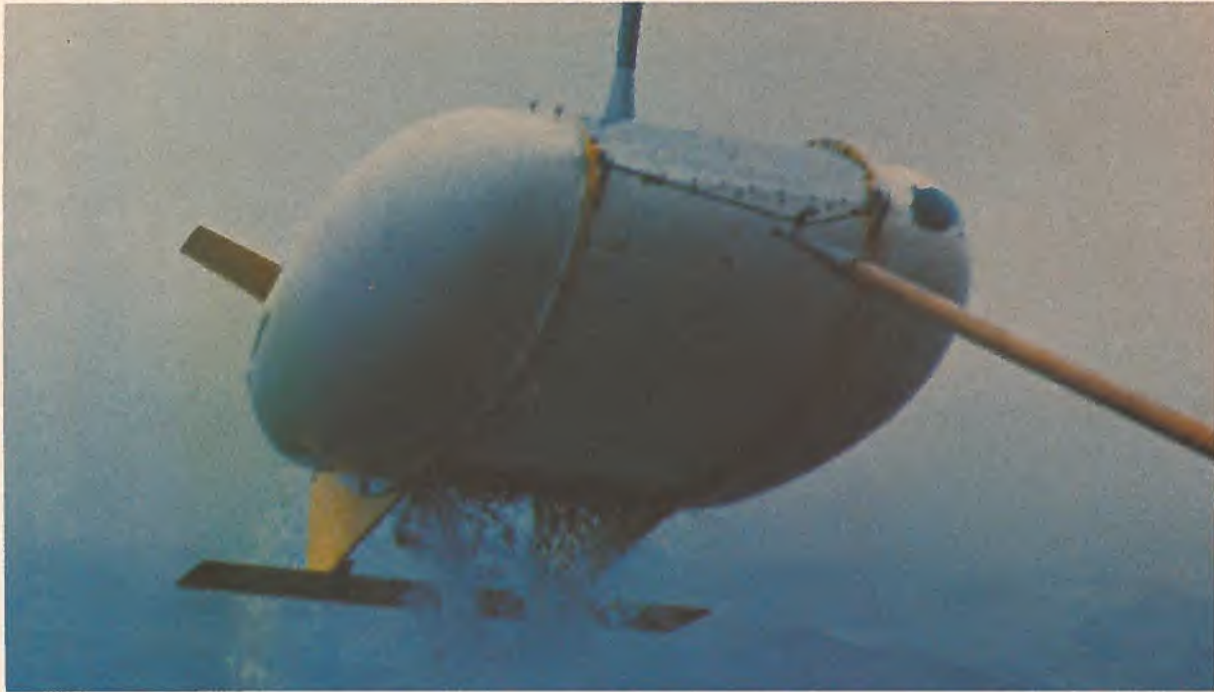
Huntec's deeptowed seismic system gives unmatched resolution of the seismic section and allows the system to operate in weather conditions that would render other equipment inoperable.
