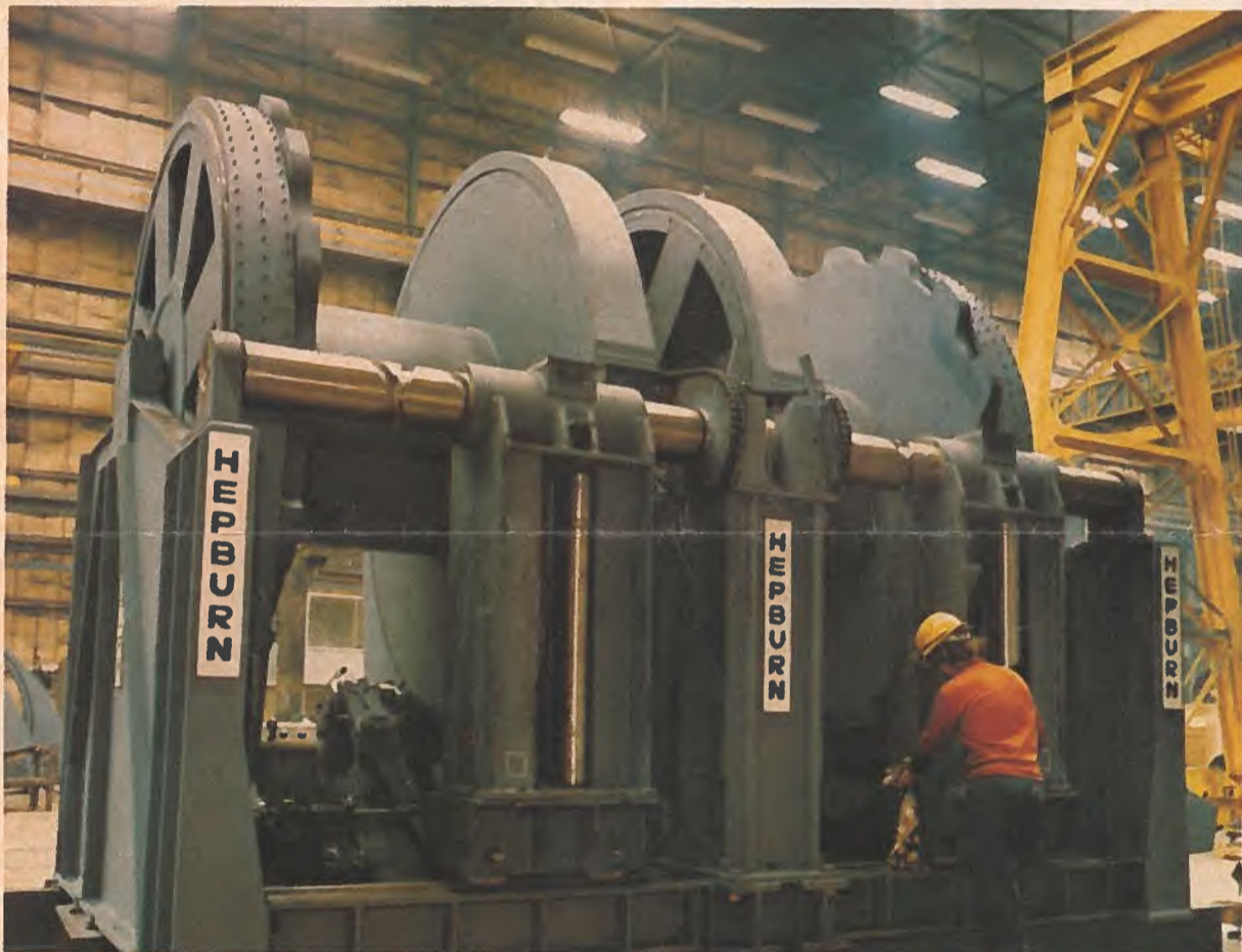
Twin-drum anchor winches by John T. Hepburn Limited are used for the accurate positioning of a drillship while drilling operations are under way.
