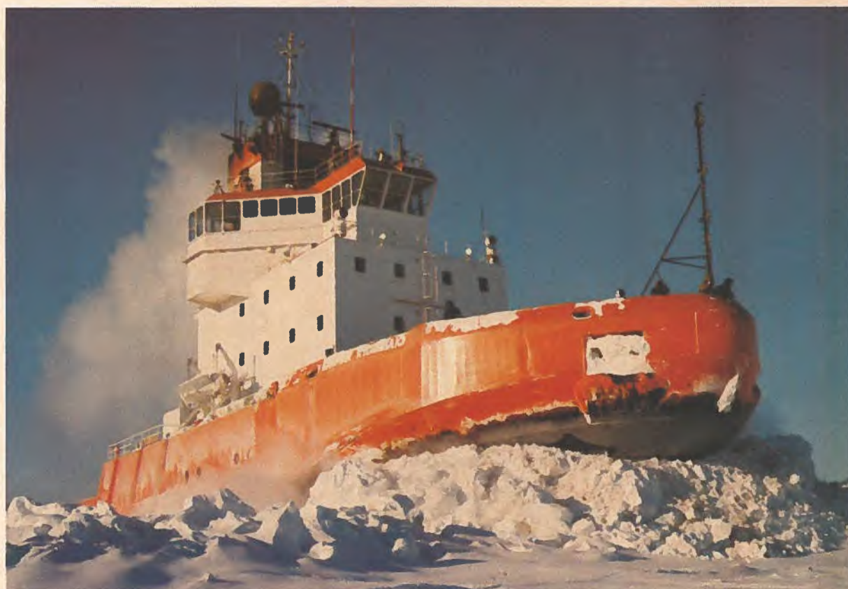
Out of Saint John Shipbuilding, the "Canmar Kigoriak", the first vessel to be built to the rigorous requirements of the Canadian Arctic Waters Pollution Prevention Regulations, Class 3.
