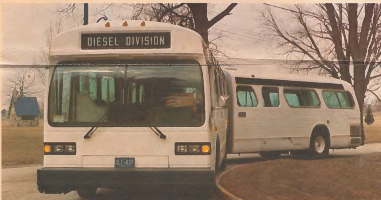
Newest addition to the General Motors of Canada Limited fleet of urban transit products is the articulated bus, an adaptation of GM's New Look transit coach affectionately known as "Old Faithful". Two New Look shells have been successfully married to form the basis of the articulated bus. They are tied together by a proven push-type turntable that: provides control over the relative lateral motion between the front and rear sections of the coach under normal driving situations; gives full damping action restricting lateral motion at highway speeds; and provides anti-jackknife protective control.
