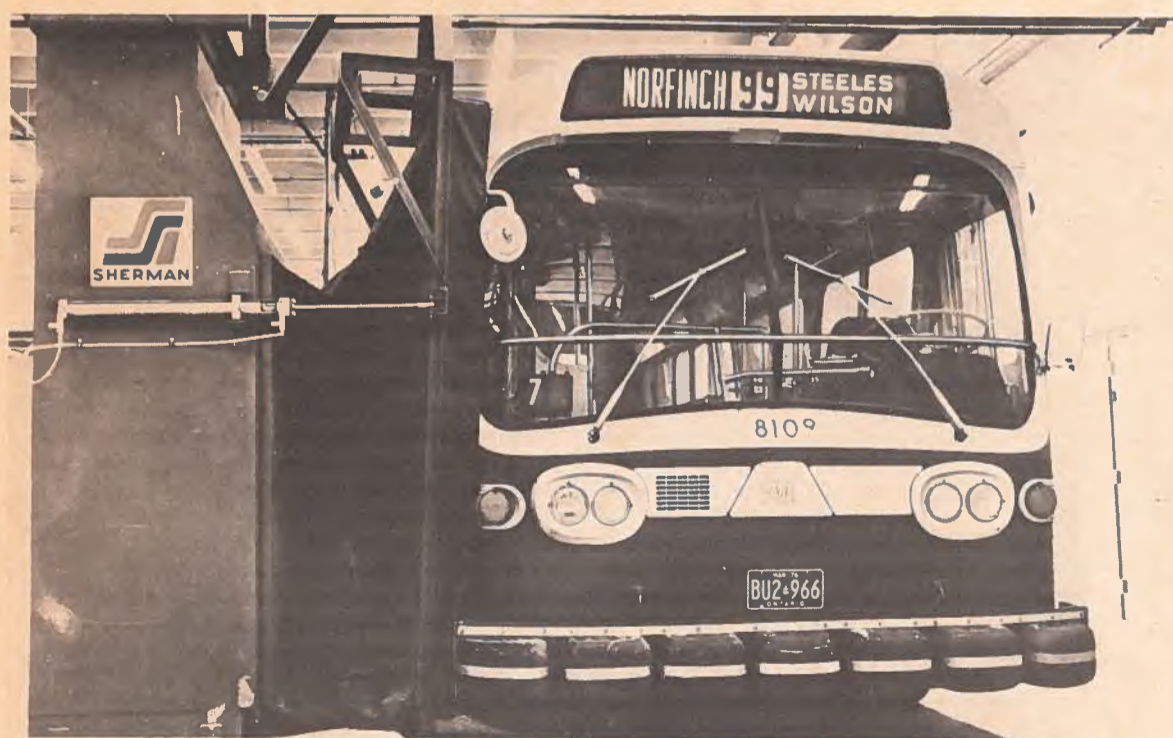
The Sherman Cyclon Bus Vacuum System cleans loose debris from a transit system bus in 2.5 minutes by agitating it from the back door and sucking it out the front door by a bellows-type vacuum system that completely seals the front door.
