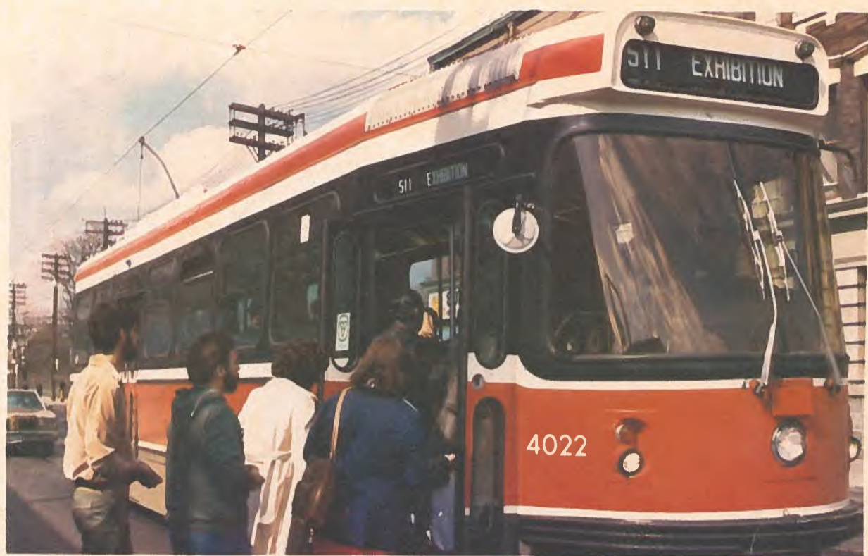
The Canadian Light Rail Vehicle was placed in service in Toronto on September 30, 1979. Developed by the Urban Transportation Development Corporation Ltd., the vehicle incorporates many new passenger comfort features including: large picture windows, fluorescent lighting, low-step entry and exit, forced ventilation and a smooth, comfortable ride.
