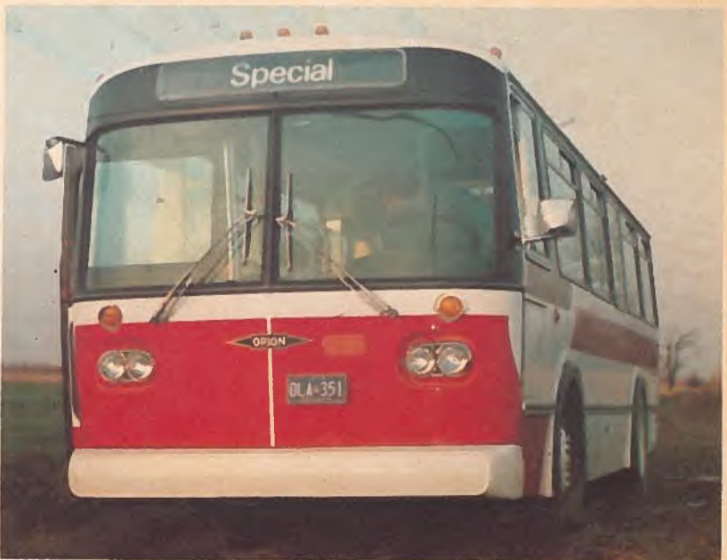
Shown in its intercity coach configuration, the 9 m (30-ft.) Orion bus has a passenger capacity of 31 to 33 seated. In transit configuration it can seat 31 with a further 30 standing. The 10 m (35-ft.) model Orion can seat 39 to 45 as a coach, and in transit configuration, seats 39 with 40 standing.
