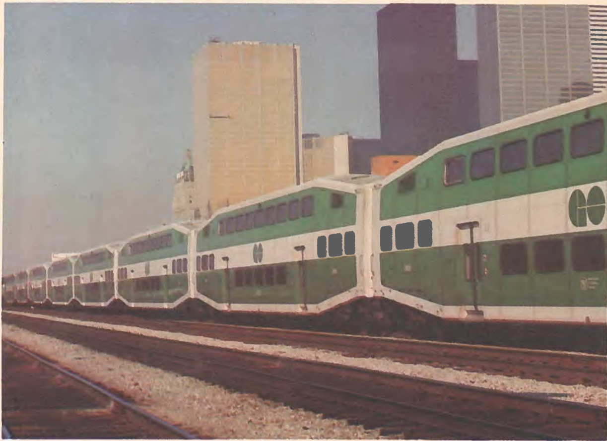
Distinctively styled bi-level coaches which seat 162 passengers on two complete decks are so successful that orders for more than 70 additional cars have been placed by GO Transit, the commuter service serving southern Ontario. Versions of this car, which can seat up to 200 passengers, are designed and built by Hawker Siddeley's Canadian Car Division.
