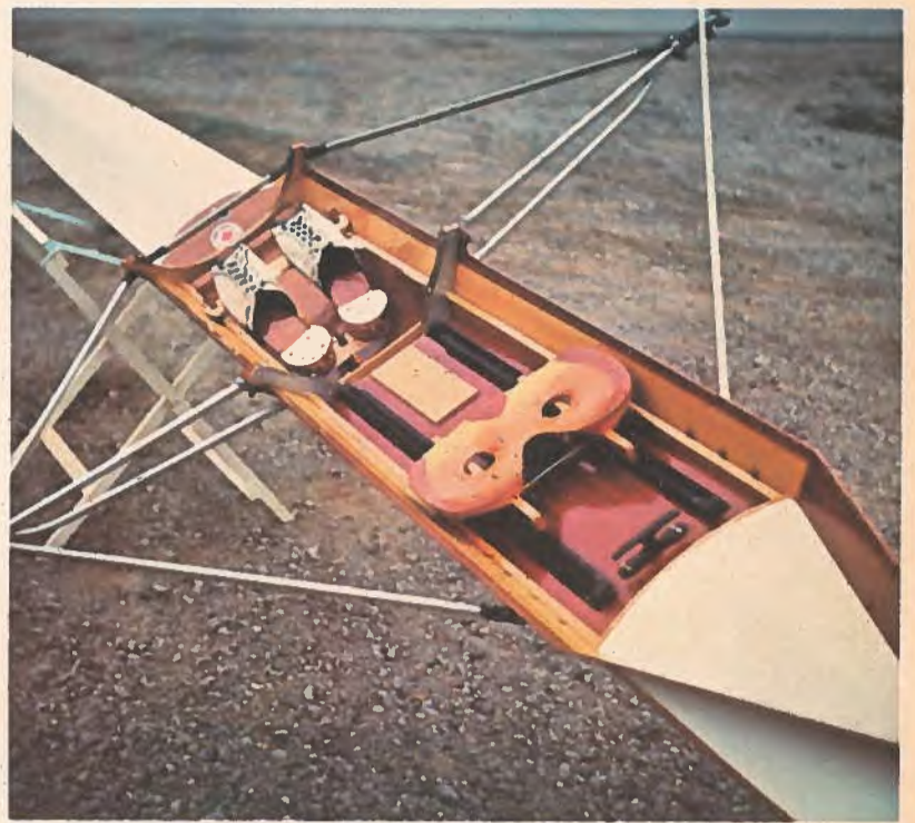
With these shoes comes one of the world's finest racing shells — made by Kaschper Racing Shells Limited in the southwestern Ontario village of Lucan. The Kaschper building method, working three wood veneers onto a special vacuum mold, assures a much stronger than normal shell with skin free of nails, screws and vulnerable joints. All competition sizes are available.
