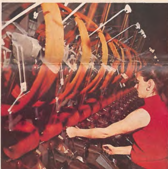
Skein-dyed knitting yarn being back-wound on a skein-to-cone winder at Cleyn & Tinker, which spins and dyes every combination of fibre and colour. This yarn will go into knitted fabric, using very latest models of knitting machine and double-jersey circular knitter. It is shipped in cones. The Cleyn & Tinker group's finished fabrics are sold in 18 countries. Code 2-5
