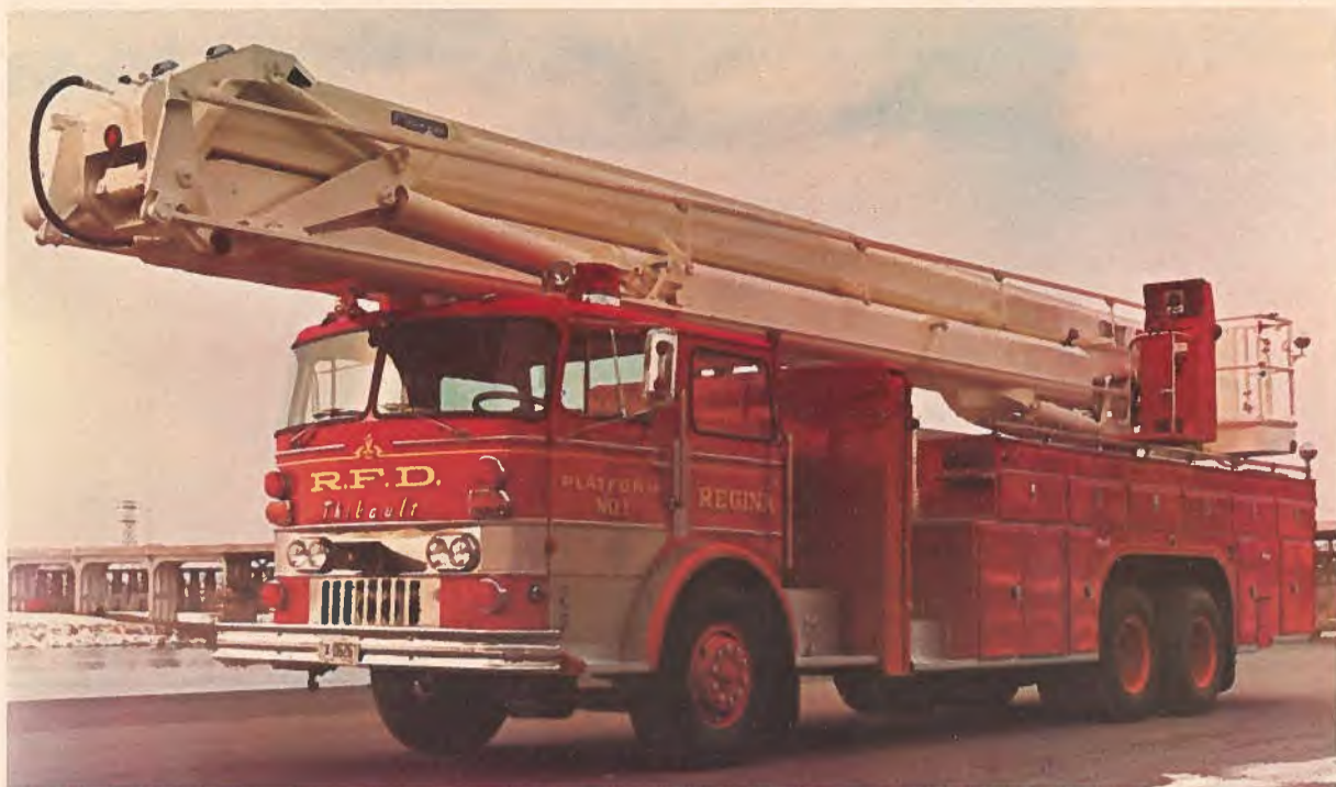
Canopy-type forward cab for firefighting, by Pierre Thibault, has ultra-modern 80-foot elevated platform. It's in use by Regina, Saskatchewan, fire department.
