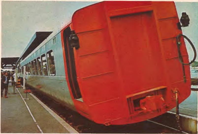
This train is tipsy? No, just tilted — so it won't lurch going around a curve. Light, swift LRC is a product of Alcan-Dofasco-MLW consortium. Code 5-2
