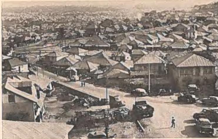
*In the old town of Ibadan, Nigeria, there is no regular street pattern and this makes it impossible to install a sewerage system of the type used in North America, as Canadian engineers soon discovered. Their solution was to set up communal facilities in strategic locations.*
