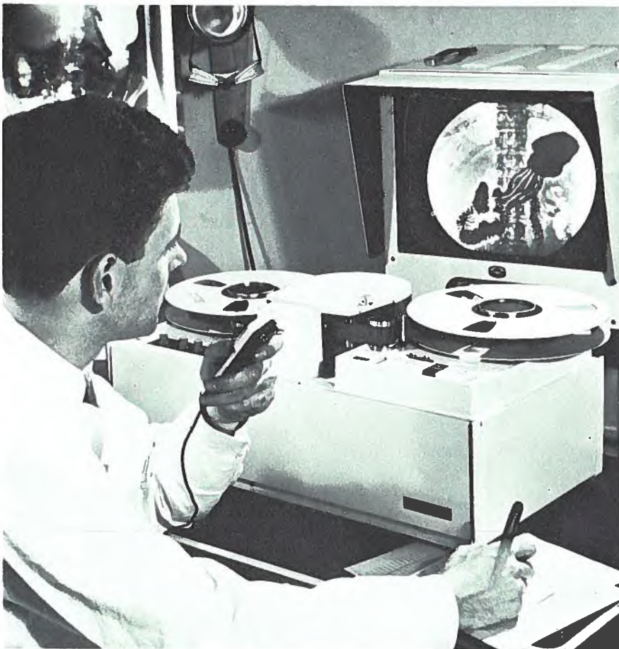
Technician monitors an X-ray examination using a transistorized X-ray picture tape apparatus connected with a picture amplifier. The equipment was manufactured locally in the Netherlands.
