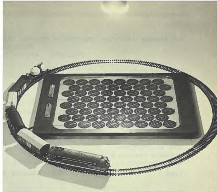
This toy electric train is not what it appears to be. It is a highly sophisticated model powered by sunlight or, in this case, by a sun-lamp shining on the cells in the tray.
