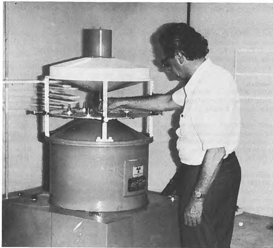
Dr. Admar Cervellini, Director of CENA, works with the Gammabeam 150 irradiator made by Atomic Energy of Canada. Note the locally made turntable. The machine is used in research and to combat disease and pests in crops.
