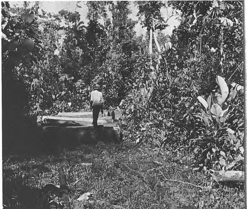
On their way to a sawmill down river, hardwood logs are rolled to the water's edge via this primitive truckway. Manual labor is the chief source of power.
