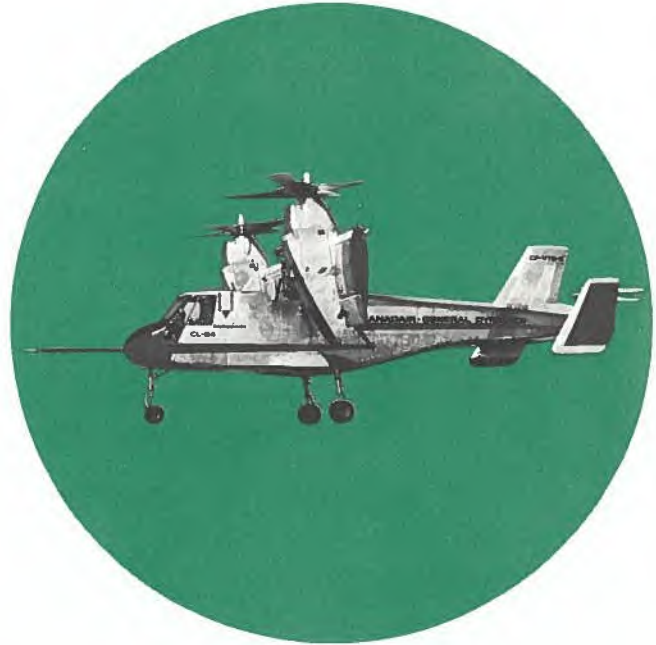
Developed with DIP program support, Canadair's CL-84 "tilt-wing" aircraft can take off vertically and hover like a helicopter then fly forward like a conventional plane at speeds up to 350 mph.
