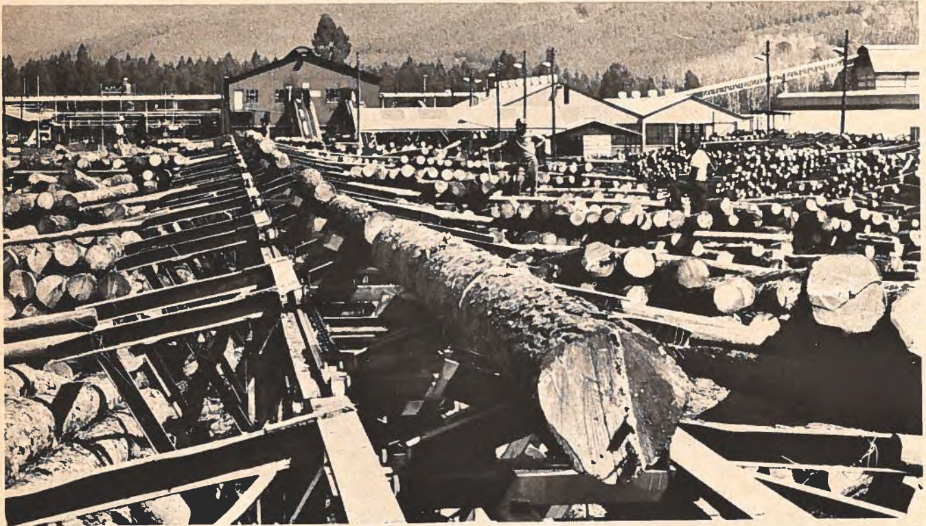
A manually operated mechanical log sorting line in the eastern Transvaal. (Photo: W.G. Winckler, S.A. Lumber Millers Assn.)
