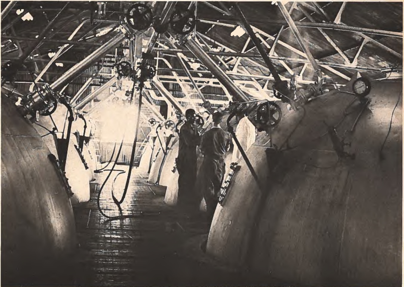
Fermentation vessels in a chemical plant in Germiston which uses sugar cane molasses.
