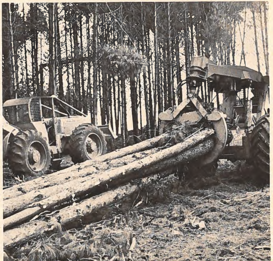
A Timberjack grapple skidder and double drum skidder. (Photo: Eaton Kent S.A. (Pty) Ltd.)
