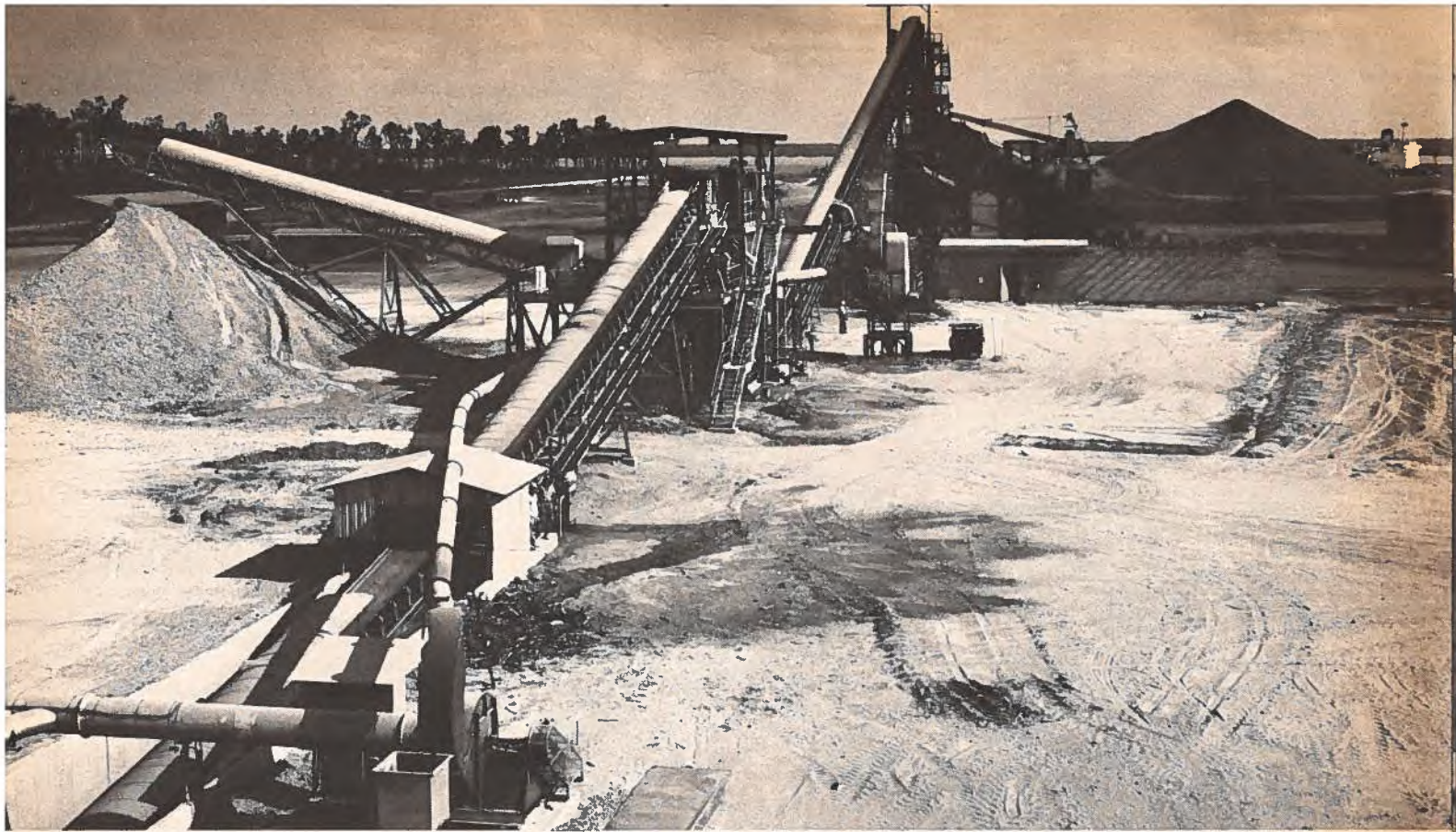
This bauxite mine on Cape York Peninsula has to remove only a few feet of soil to find the ore body that varies in thickness from a few feet to 30 feet.
