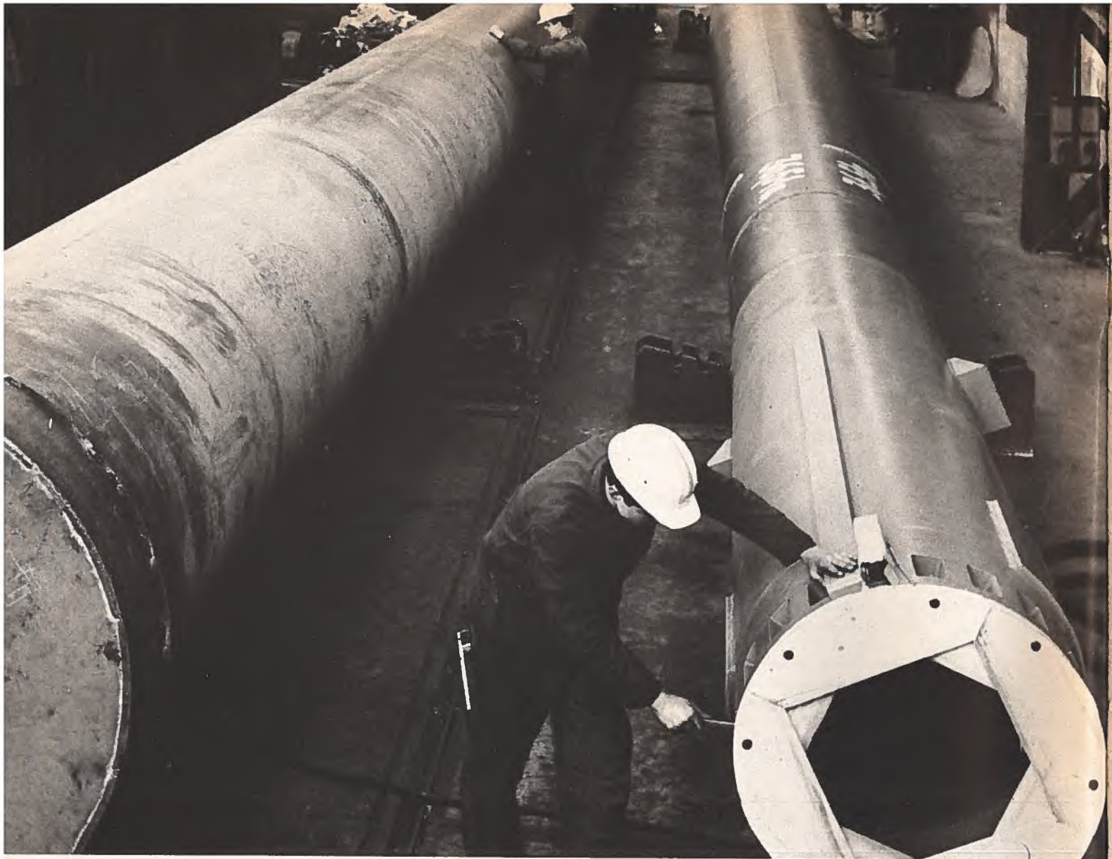
Steel-tube mooring posts in the final stage of manufacture at Mannesmann AG.
