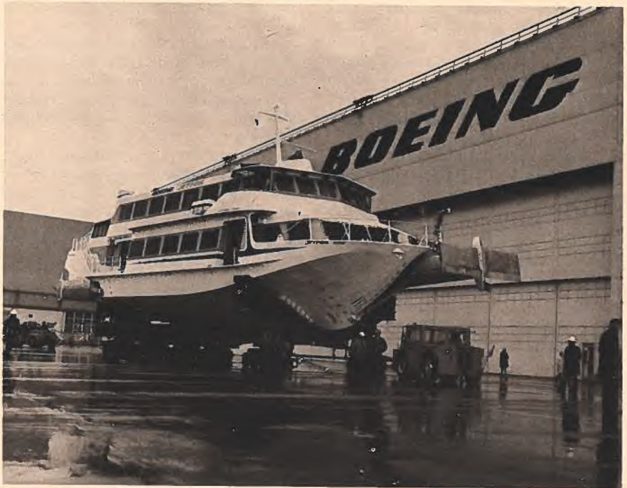
... and this Jetfoil 929 designed to carry 250 passengers at a cruising speed of 50 m.p.h. over 12-foot-waves, are also Boeing products.
