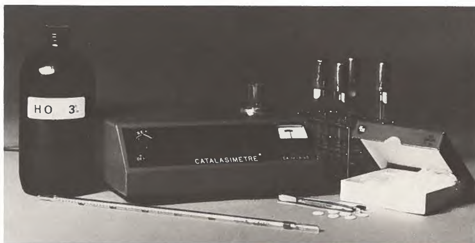
The Catalasimetre — an instrument for the rapid estimation of the amount of the enzyme "catalase" present in aqueous solutions — developed by the Centre des recherches en sciences appliquées à l'alimentation (CRESALA) and now manufactured by Allca Instruments Cie Ltée.
