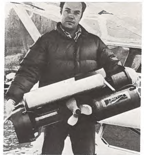
A winner at the Houston offshore technology conference was the Dart, International Submarine Engineering's latest submersible and perhaps the world's smallest self-propelled TV monitoring system.
