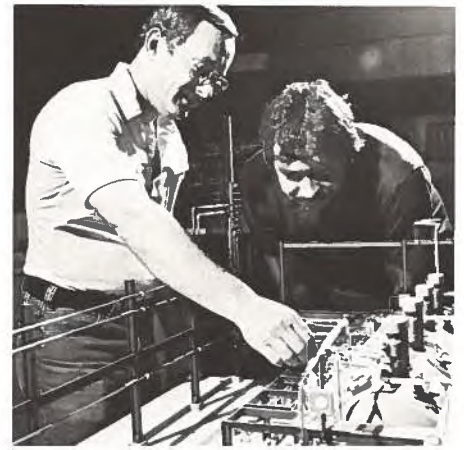
This engineering model helps Cominco staff visualize the placement of equipment on the full-scale zinc pressure leaching facility being constructed outside their engineering offices at Trail.
