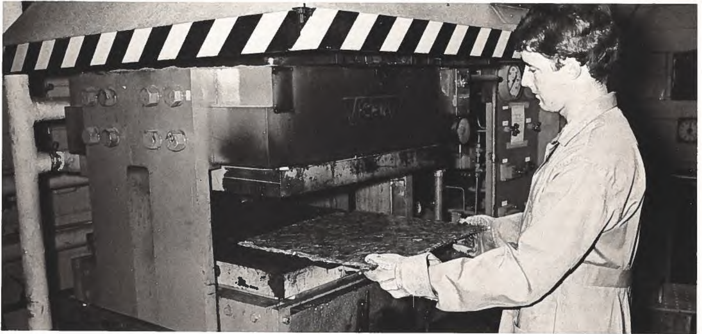
Hand sheets of waferboard are made in the Forintek laboratory using lignin-based adhesives. These new, inexpensive adhesives are made from pulp mill wastes.
